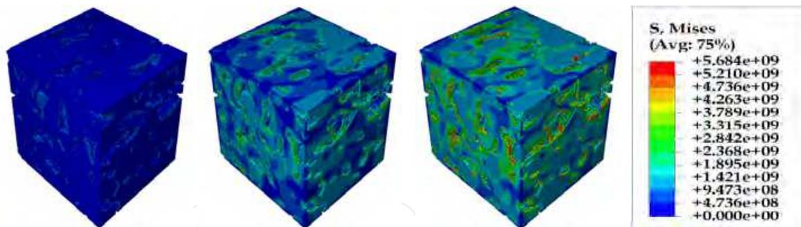
Fig. 8. Von Mises stress contour plots for anode considering elastic-plastic behavior of nickel: (left to right)  $\Delta T = 100^\circ\text{C}$ ,  $\Delta T = 500^\circ\text{C}$ ,  $\Delta T = 800^\circ\text{C}$
