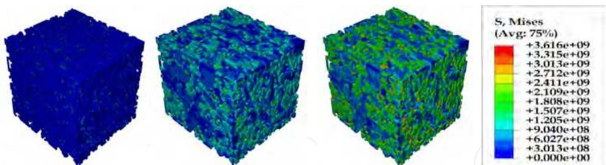
Fig. 9. Von Mises stress contour plots for cathode considering temperature-dependent material properties: (left to right)  $\Delta T = 100^\circ\text{C}$ ,  $\Delta T = 500^\circ\text{C}$ ,  $\Delta T = 800^\circ\text{C}$
