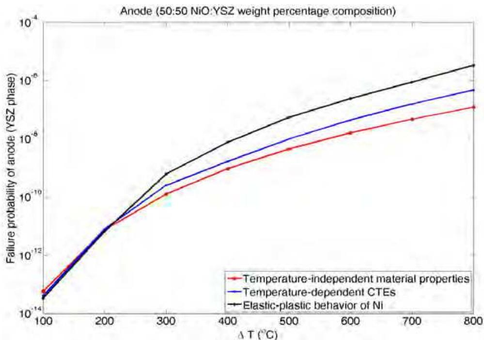
Fig. 10. Probability of failure values for anode
