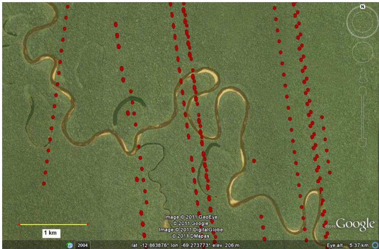
Fig. 3. Multiple GLAS laser campaigns sampling overlaid on a GoogleEarth image of Tambopata, Peru. Missing data are found where dense cloud prevents sufficient energy from penetrating to the Earth's surface and returning to the sensor.
