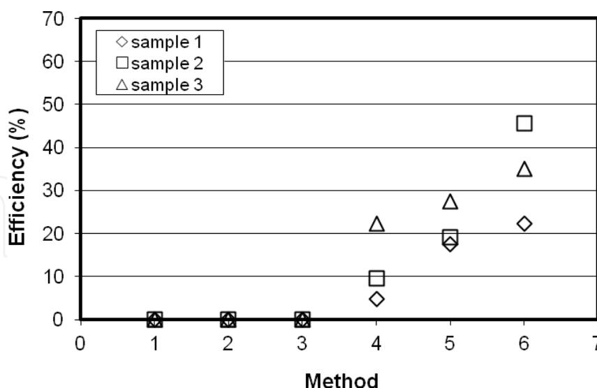
Fig. 14. The method efficiency of 0.5 Bq/mL urine sample preparation. Number 1 represents the F method, numbers 2-6 represent the A – E method.
