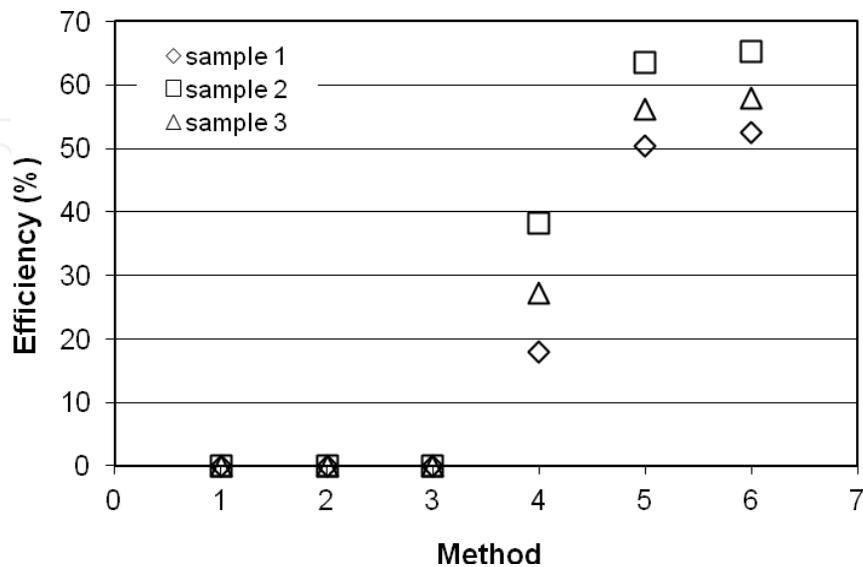
Fig. 15. The method efficiency of 1 Bq/mL urine sample preparation. Number 1 represents the F method, numbers 2-6 represent the A - E method.
