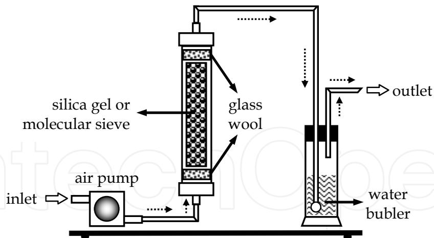
Fig. 1. The apparatus for tritiated water vapor sampling
