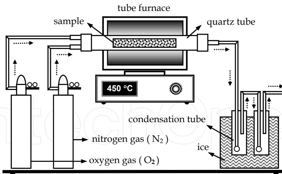
Fig. 6. The apparatus for soil samples preparation
