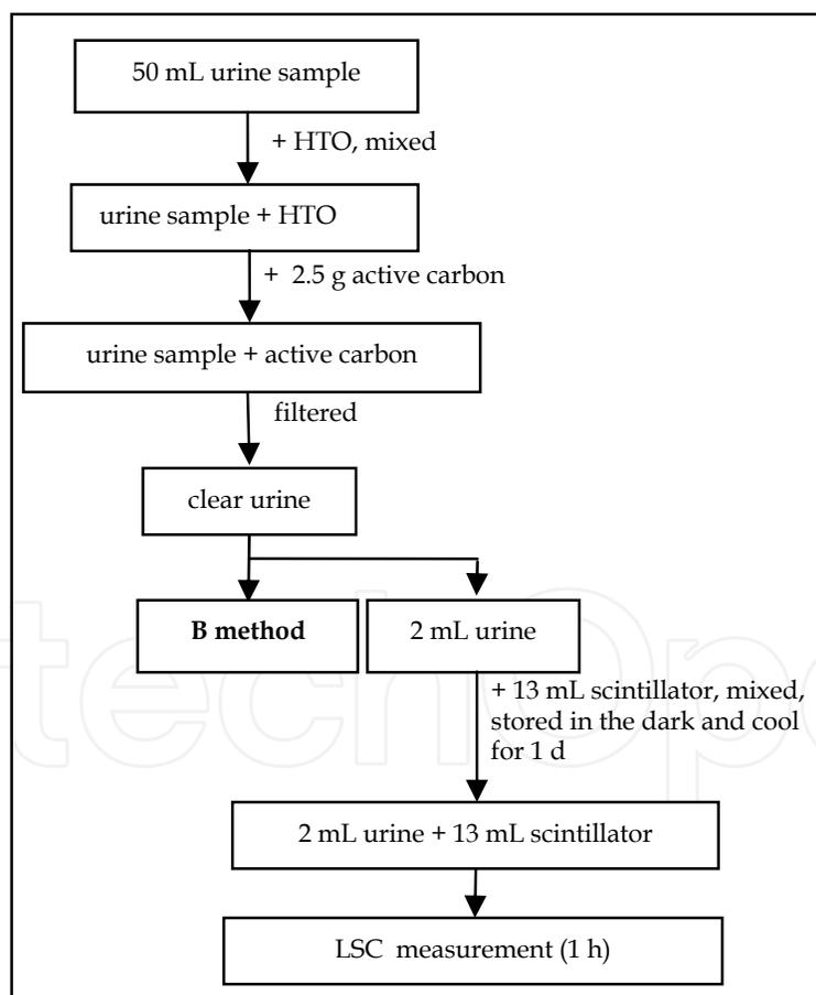
Fig. 9. The scheme of urine sample preparation by A method
