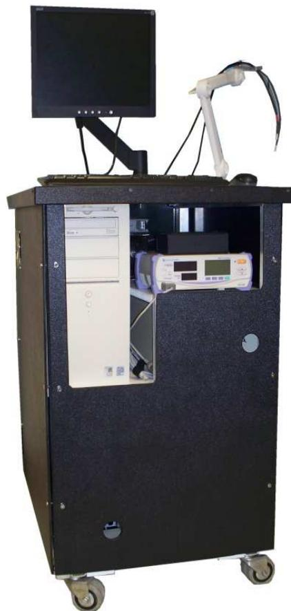
Fig. 2. Picture of the portable NIRS apparatus.
