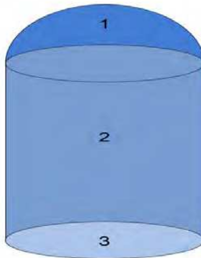
Fig. 13. Volume composed of a cylinder and a spherical cap used to find the radiative transfer among those surfaces
