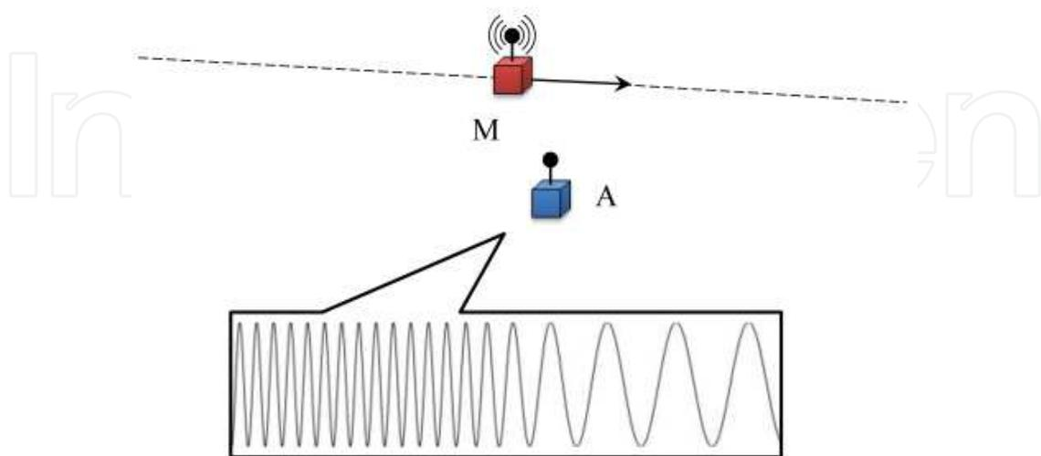
Fig. 5. Illustration of the Doppler frequency shift in the signal introduced by the relative velocity of the moving transmitter to the stationary receiver.
