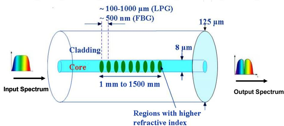
Fig. 1. Schematic representation of a fiber grating
