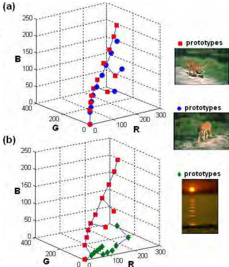
Fig. 3. WW-test for a pair of similar images (a) and dissimilar images (b), based on the  $k=12$  color prototypes shown in Fig. 2. In the top panel, there are 19 edges having differently labeled nodes as endpoints and therefore splitting the overall MST into 20 subgraphs, thus  $R=20$  ( $W=2.6523$ ). On the contrary there are only 2 such edges in the bottom panel, thus  $R=3$  ( $W=4.8361$ ).
