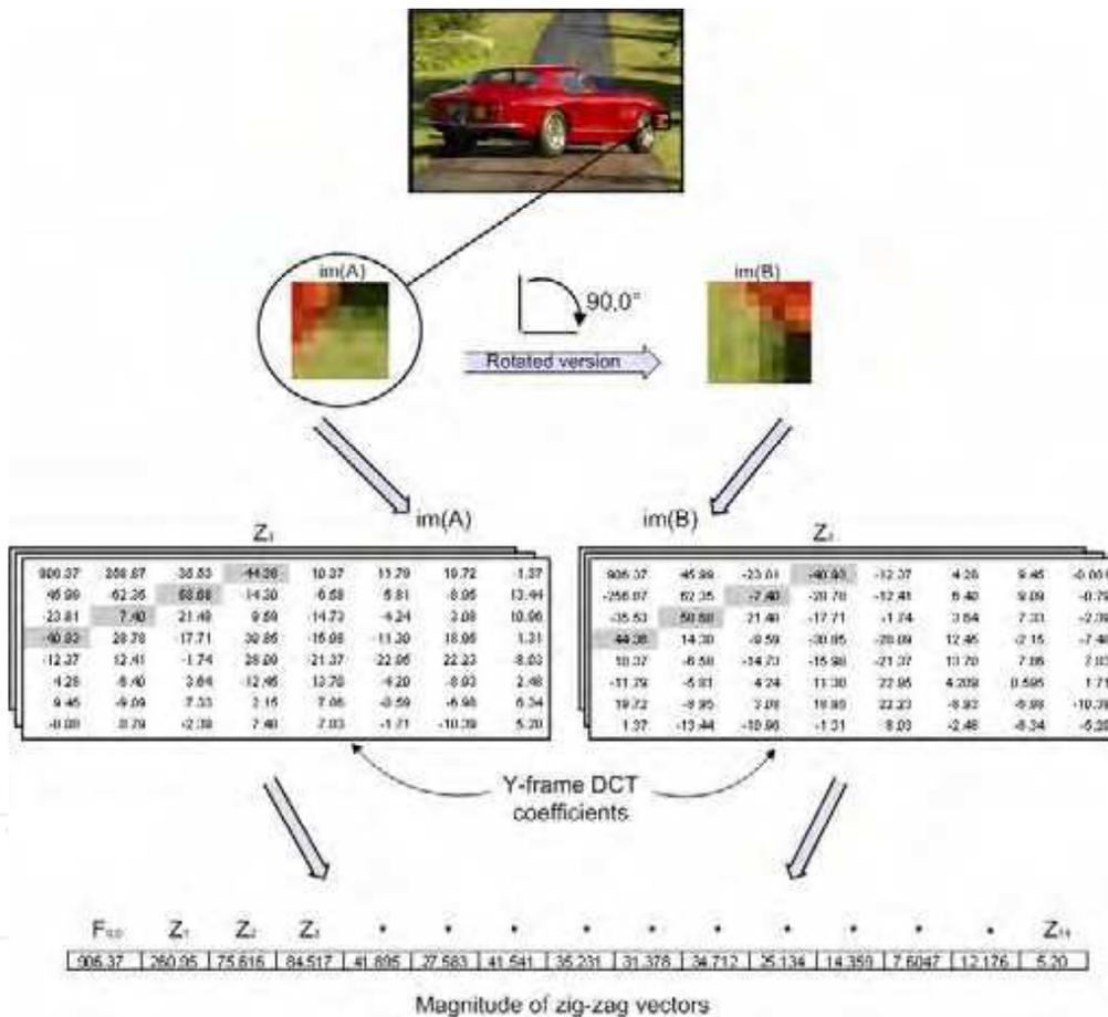
Fig. 6. DCT coefficients in the case of an image macroblock  $im(A)$  and its rotated version  $im(B)$ . Each diagonal line of the zig-zag scheme is considered as a vector. The corresponding vectors (gray-shaded) contain AC coefficients having equal absolute value, although they are located at different positions. However, their magnitudes are the same, as provided at the bottom panel.
