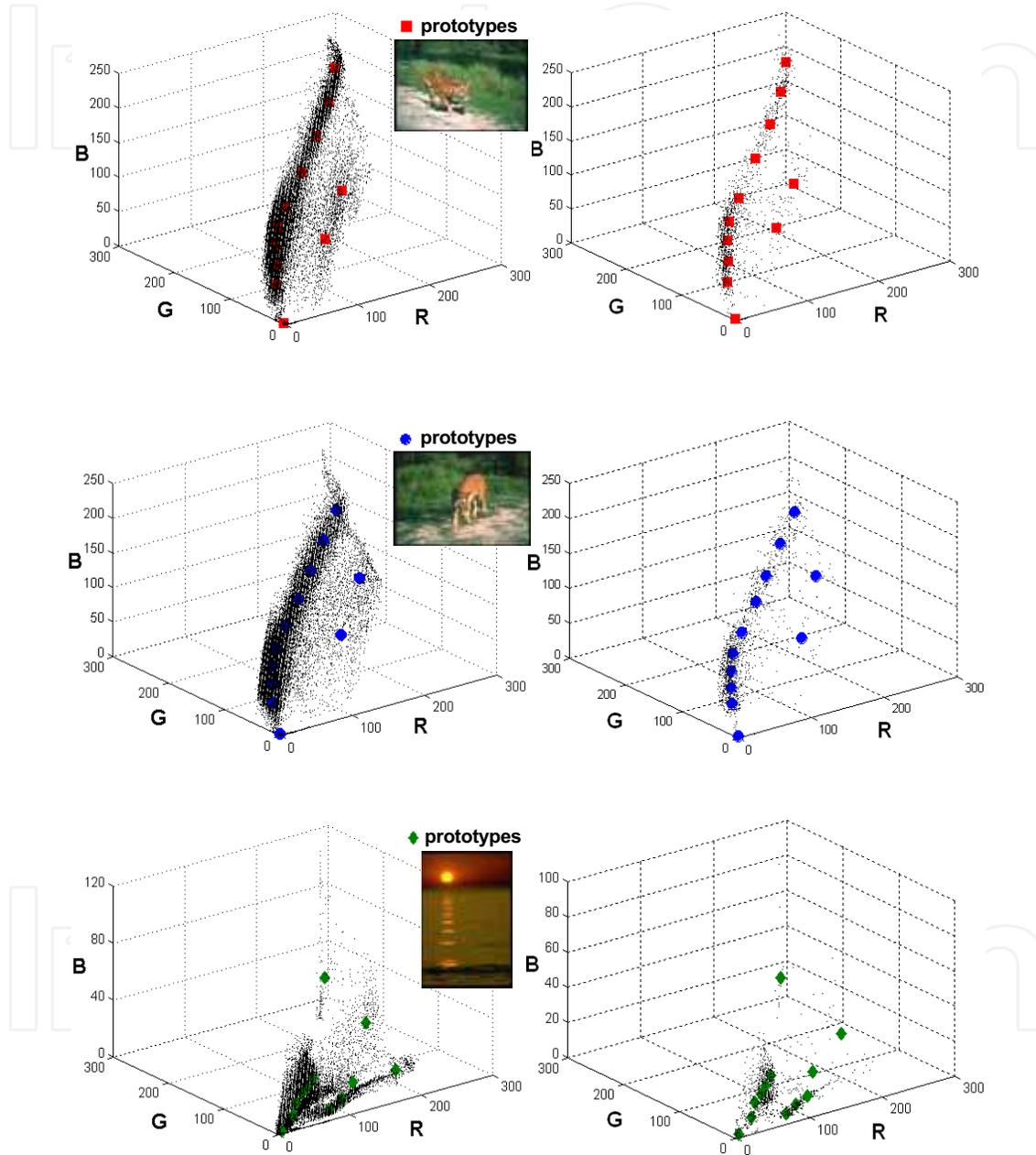
Fig. 2. Codebook color representation based on the Neural-Gas algorithm. For each image, a point-distribution is formed using the RGB-vectors corresponding to all (left panel) or a small portion (right panel) of the pixels, summarized through 12 prototypes.
