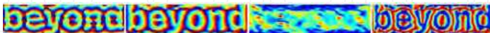
Fig. 8. Log-Gabor filtering results for each filter property. From left to right: phase of the horizontal filter, phase of the vertical filter, magnitude of the vertical filter and absolute phase of the vertical filter.
