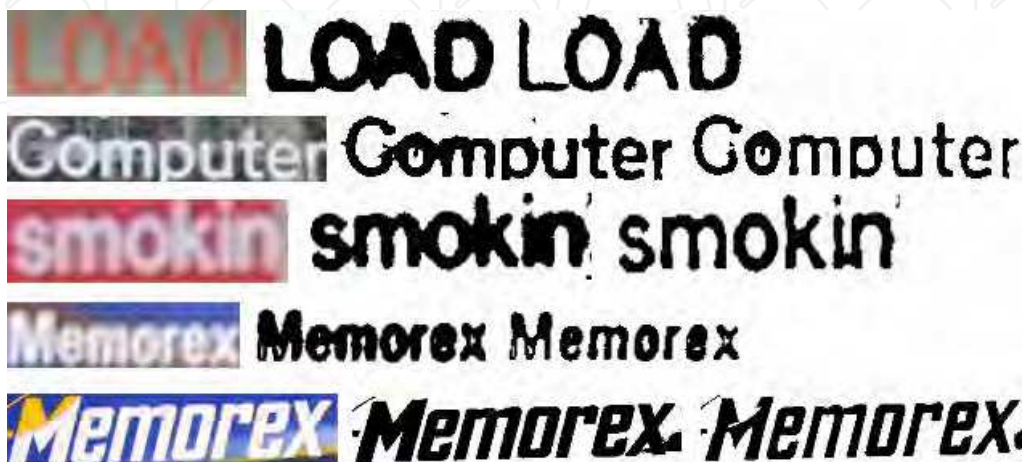
Fig. 10. Some character segmentation examples. From left to right: original image, SMC-based binary version and result after character segmentation.
