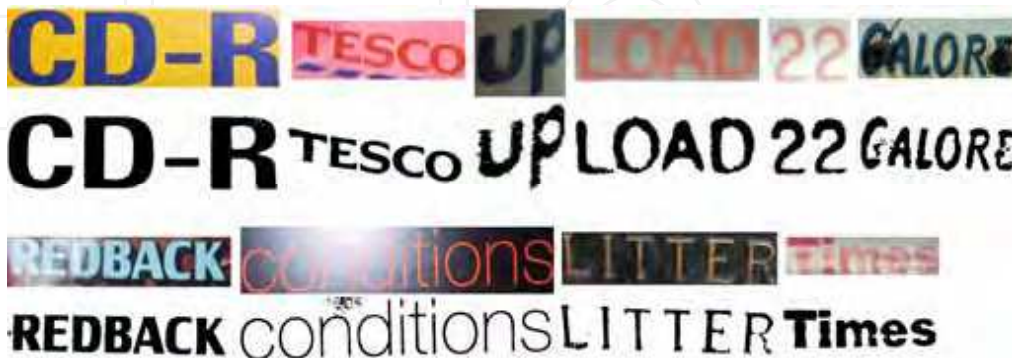
Fig. 5. Extraction results using SMC in a RGB-based k-means framework.
