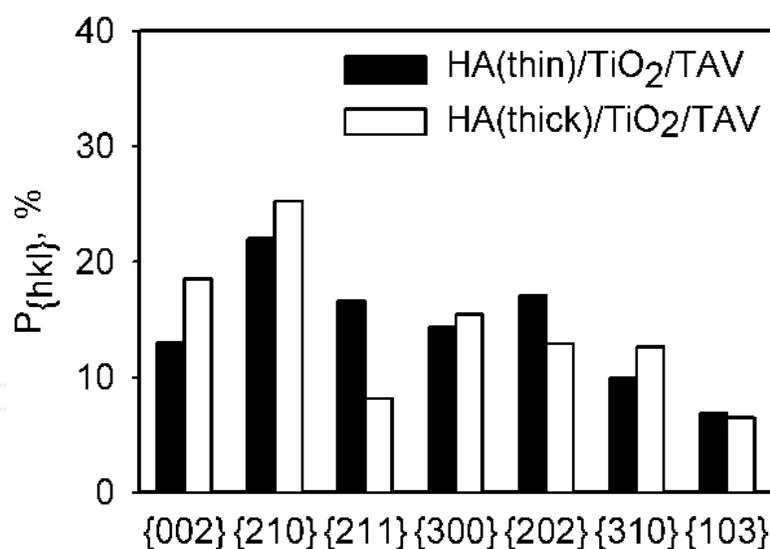
Fig. 6. Pole density histograms, representing the share of HA crystallites, oriented with their  $\{hkl\}$  planes parallel to the substrate surface in two double-layer plasma-sprayed coatings (thin and thick) with transition  $\text{TiO}_2$  and top HA layers (Gueorguiev et al., 2009b).
