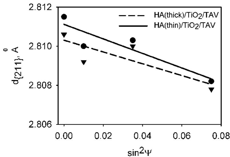
Fig. 8. Experimental data and least square linear fits of the dependencies of the interplanar HA spacing  $d_{\{211\}}$  versus  $\sin^2\psi$  for two double-layer plasma sprayed coatings with transition TiO<sub>2</sub> and top HA layers differing in thickness (Gueorguiev et al., 2009b).
