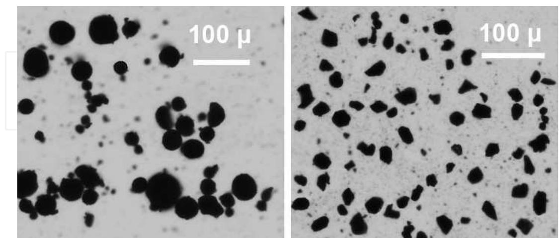
Fig. 2. Particles of powders XPT-D-703 (HA, left) and AMDRY-6505 (TiO<sub>2</sub>, right), observed in transmission optical microscope (Gueorguiev et al., 2008a, 2008b).
