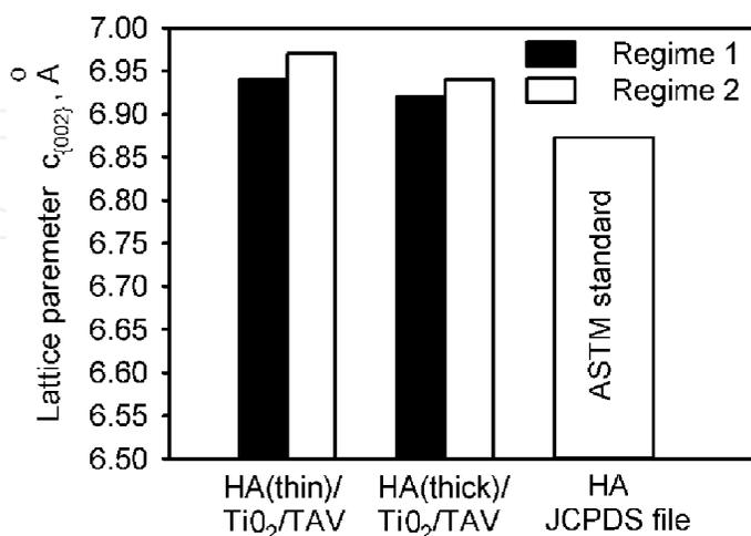
Fig. 7. Lattice parameters  $c_{\{002\}}$  for the HA layer in two double-layer plasma-sprayed coatings with transition TiO<sub>2</sub> and top HA layers, differing in spraying regime and thickness, together with the respective standard JCPDS value (Gueorguiev et al., 2008c).
