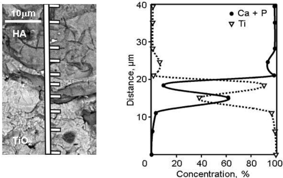
Fig. 3. SEM image (BSE mode) of the interface between the transition  $\text{TiO}_2$  and top HA layers of a plasma-sprayed bioceramic coating (left) together with the corresponding EDX profile of Ca, P and Ti concentrations (right) (Gueorguiev et al., 2009b).
