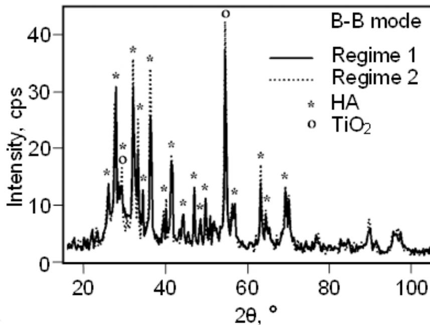
Fig. 5. XRD patterns registered in B-B mode from two double-layer bioceramic coatings with transition  $TiO_2$  and top HA layers, deposited on TAV substrates in two different plasma-spraying regimes (Gueorguiev et al., 2008c).
