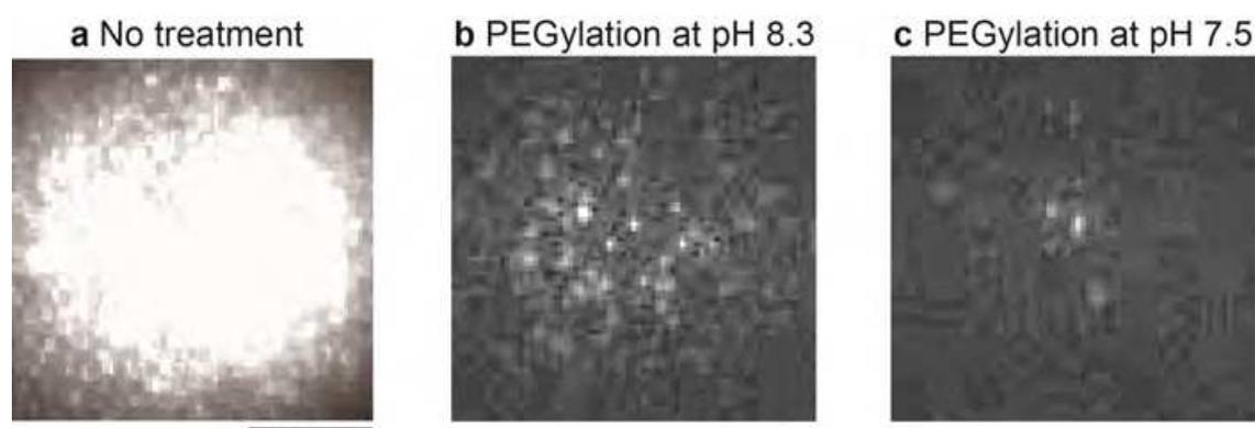
Fig. 2. Enhancement of protein-non-adsorption capability on silicate coated with PEG dissolved in 50 mM MOPS (pH 7.5). Fluorescence images of Cy5-UvrD non-specifically adsorbed on silicate with (a) no treatment, coated PEG dissolved in (b) 0.1 M sodium bicarbonate (pH 8.3) and (c) 50 mM MOPS (pH 7.5). The Cy5-UvrD concentration used was 2 nM. Scale bar, 10  $\mu$ m.
