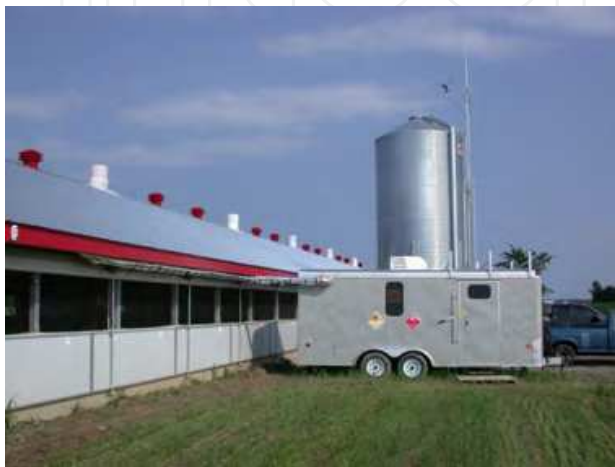
Fig. 2. View of an emission measurement set up on a naturally ventilated barn.
