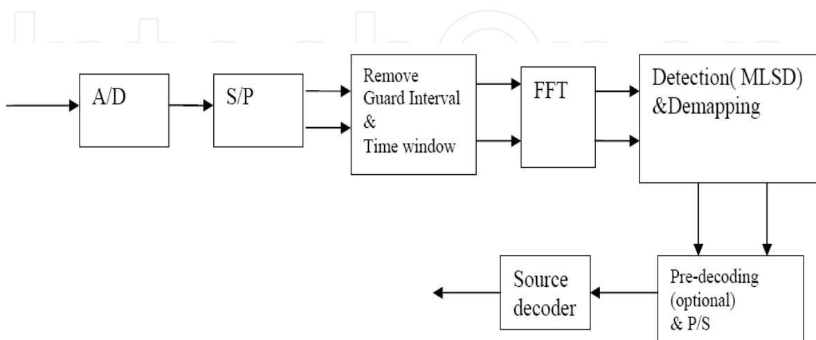
Fig. 9. Receiver block diagram of the carrier-by-carrier PRS OFDM [Naghsh & Omid, 2010]
