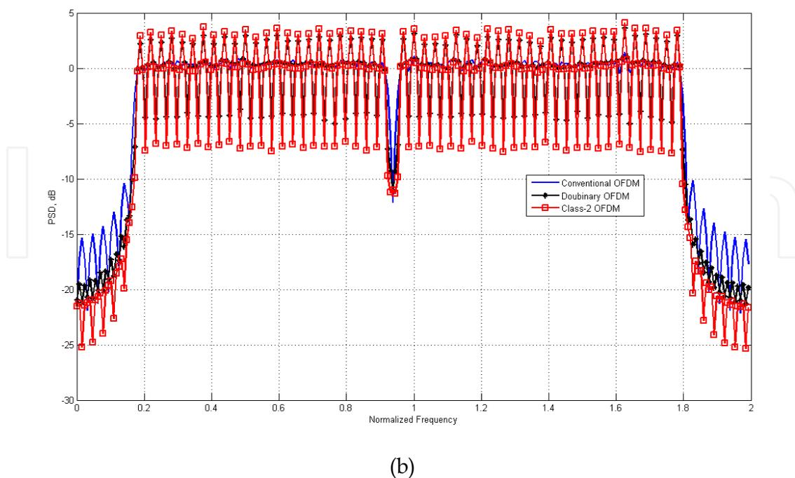
Fig. 11. a) A subcarrier, b) Overall PSD; comparison of conventional, Duobinary, and a class-2 carrier-by-carrier PRS OFDM
