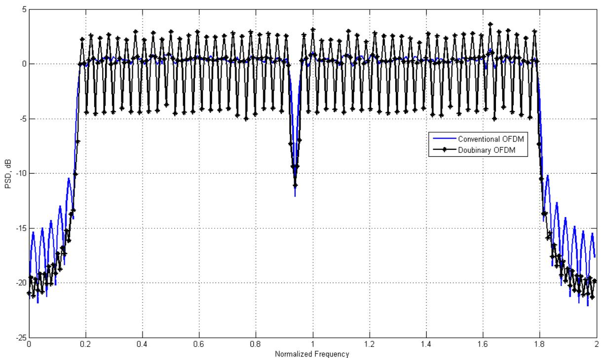
Fig. 10. PSD comparison of conventional and Duobinary carrier-by-carrier PRS OFDM for 802.11a
