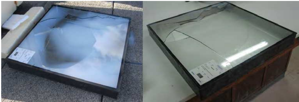
Fig. 1. Brittle fracture of panels tested in the laboratory of the Department of Construction and Technology in Architecture, School of Architecture. (UPM.) E.T.S.A.M.
