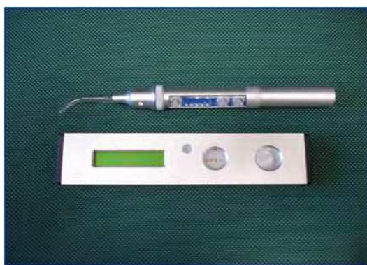
Fig. 8. Fiber-optic transillumination device (DioPower Lamp)
