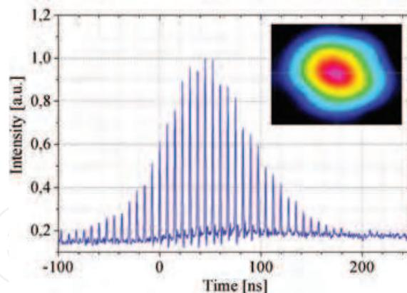
Fig. 14. Output pulse train without cavity dumping.
