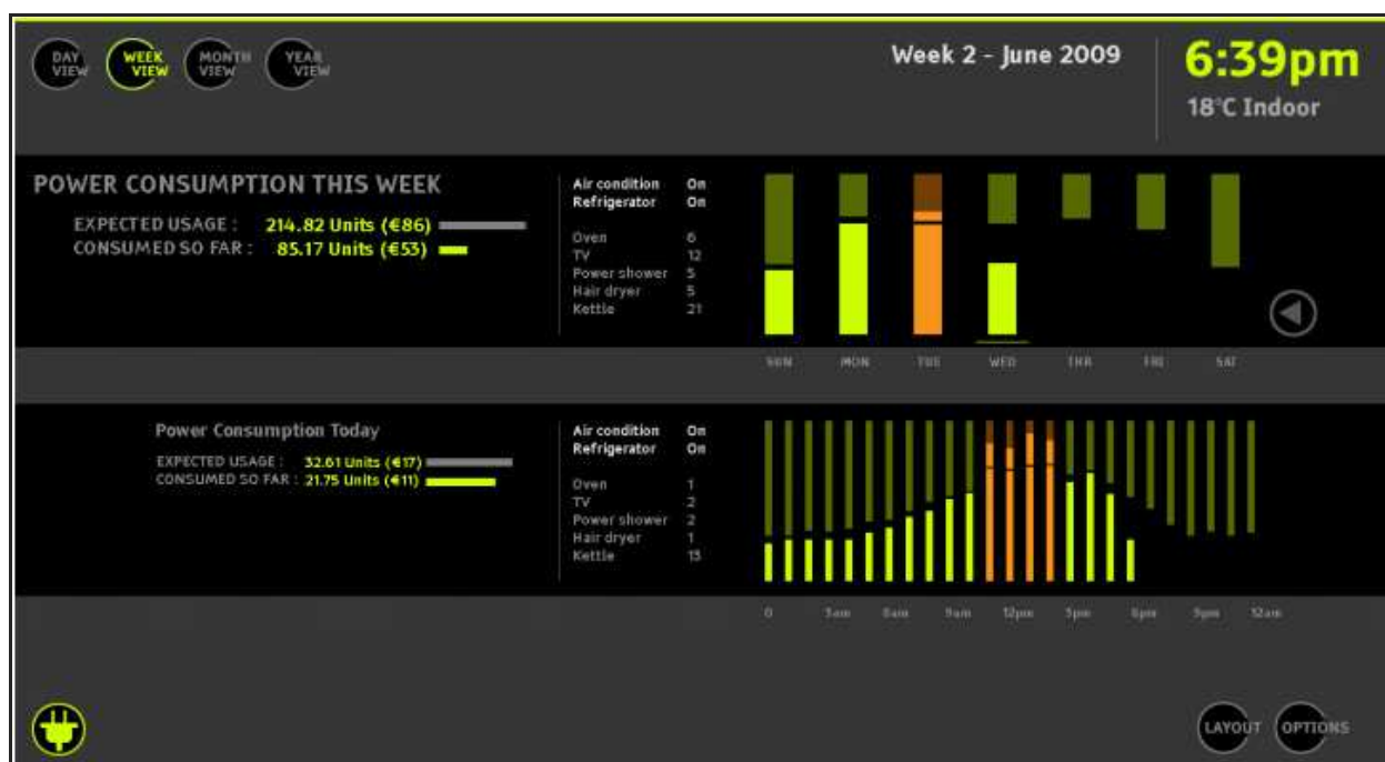
Fig. 5. Example of dark background with bright information; In-home display electricity monitor, Doherty et al. (2010).
