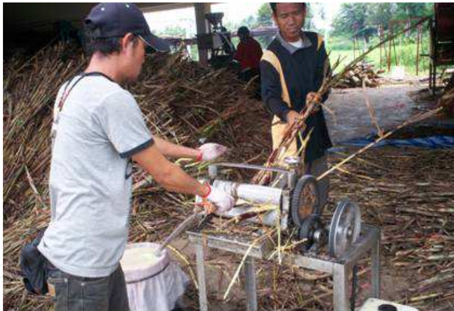
Fig. 3. Stems of sweet sorghum are squeezed by a roller mill for preparing sweet sorghum juice (SSJ)
