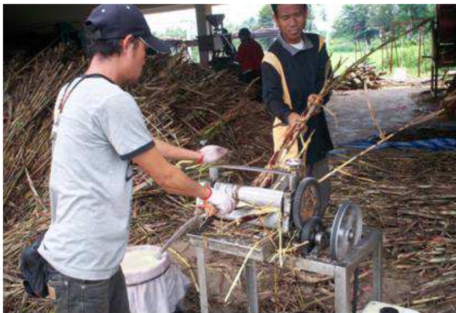
Fig. 3. Stems of sweet sorghum are squeezed by a roller mill for preparing sweet sorghum juice (SSJ)
