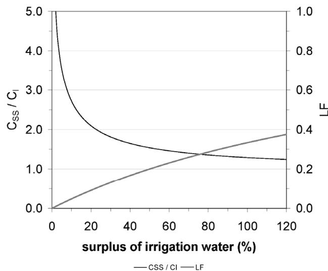
Fig. 2. Leaching fraction (LF) and relative salinity of the soil solution ( $C_{SS} / C_I$ ) as function of the surplus of irrigation water following a 40:30:20:10 root water uptake pattern and a quotient  $R / ET_c$  of 0.5. Equations after Hoffman & Van Genuchten (1983)
