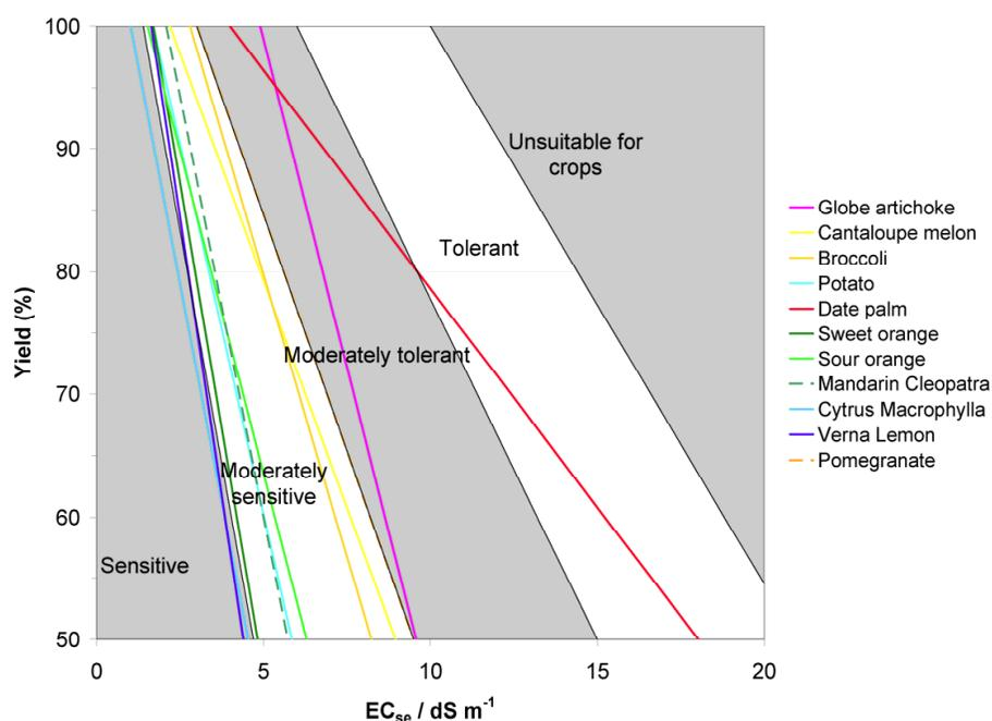
Fig. 4. Threshold-slope functions of yield versus electrical conductivity of the soil saturation extract ( $EC_{se}$ ) for the crops simulated with SALTIRSOIL\_M in the *Vega Baja del Segura*. Categories after Maas & Hoffman (1977)
