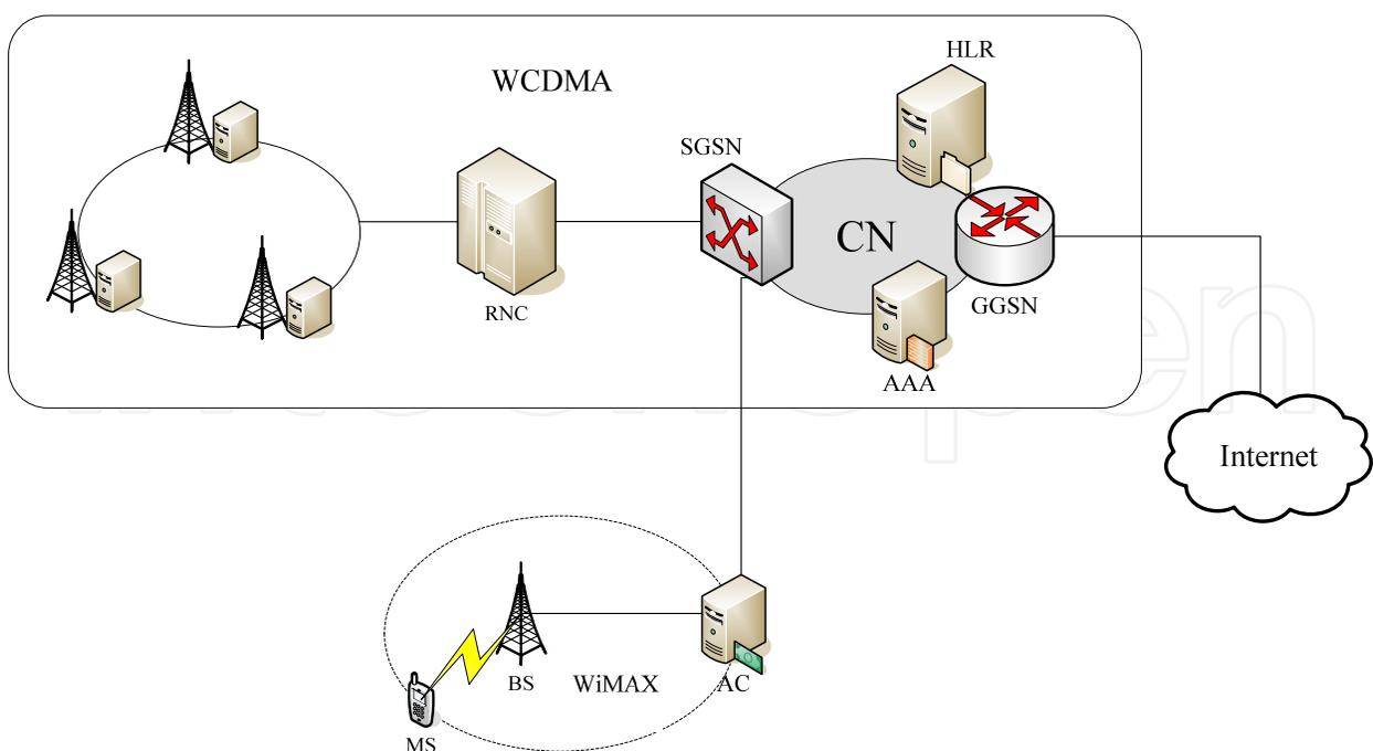
Fig. 7. Second Plan for Interoperability with 3GPP networks
