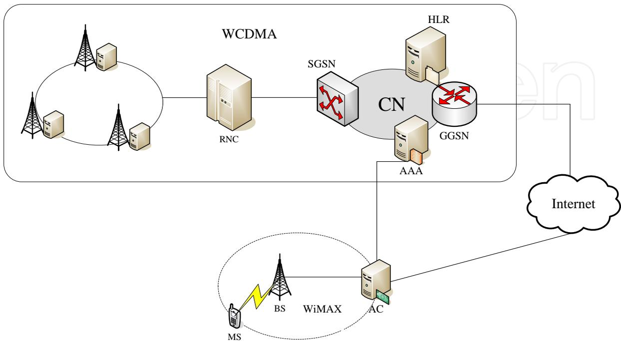
Fig. 6. First Plan for Interoperability with 3GPP networks
