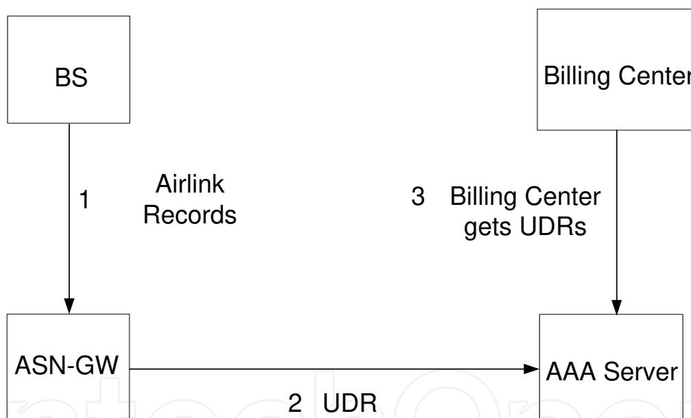
Fig. 8. Accounting Structure of WiMAX access layer
