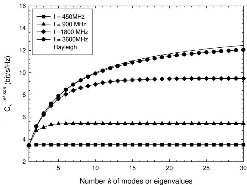
Fig. 13. Capacity  $C_k^{ref sce}$  for the reference scenario versus the number  $k$  of eigenvalues or modes taken into account. The distance between Tx and Rx is 500 m, the tunnel being 5 m wide and 4 m high (Molina-Garcia-Pardo et al., 2009b).
