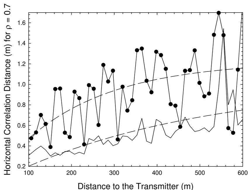
Fig. 10. Horizontal correlation distance (for  $\rho = 0.7$ ) for two tunnels for a frequency of 900 MHz. Curve with successive points deals with the tunnel 8 m wide, the other curve corresponds to the tunnel 4.5 m wide, the dashed lines give the averaged values (Molina-Garcia-Pardo et al., 2008a).
