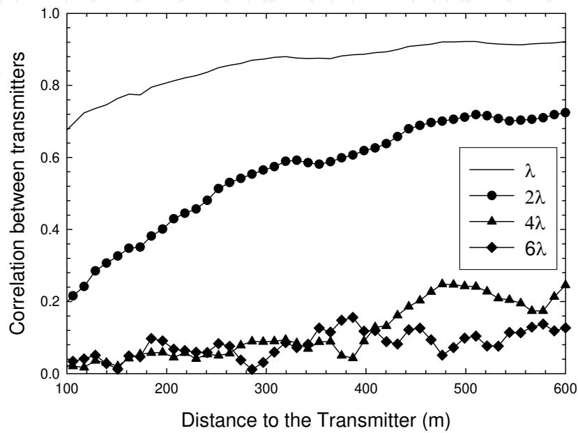
Fig. 11. Average correlation between the electric fields produced by two transmitters in the large tunnel for different array element spacing ( $6\lambda$ ,  $4\lambda$ ,  $2\lambda$  and  $\lambda$ ) (Molina-Garcia-Pardo et al., 2008a).
