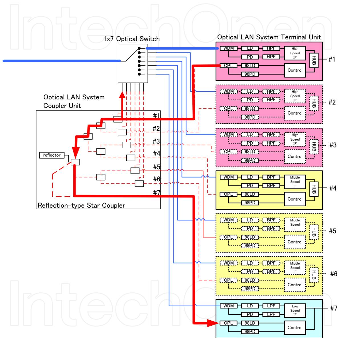
Fig. 14. Operation of communication between one “Optical LAN System Terminal Unit” and an “Optical LAN System Telephone Office Unit” using 980 nm light.
