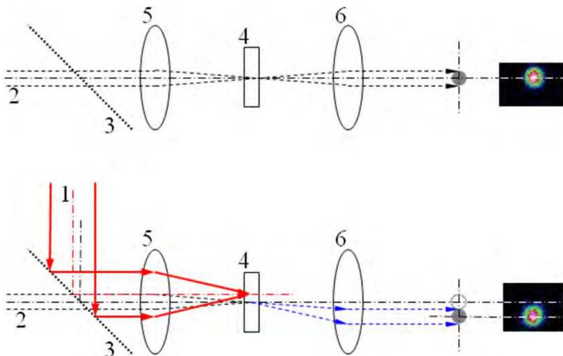
Fig. 3. Basic operation of a different axis configuration. Gating light (1) is mixed with the signal light (2) using a dichromic mirror (3), and is introduced into a dye cell (thermal-lens forming element)(4) via a focusing non-spherical lens (5). The gating light and the signal light have different axis configurations. The switched light is collimated by a lens (6). In the case with gating light, the switched light is projected to a shifted position.
