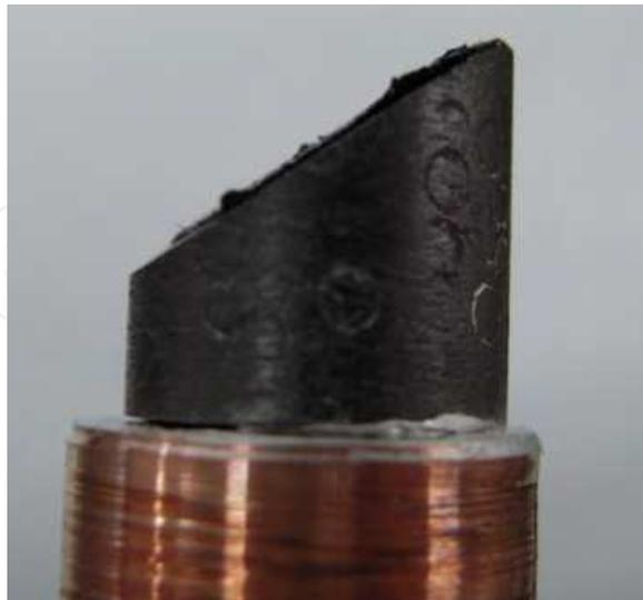
Fig. 11. Graphite anode as specimen holder.
