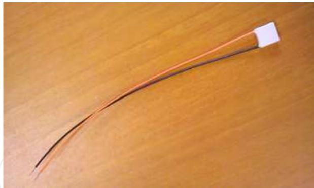
Fig. 9. Peltier device of size 8 mm × 8 mm.
