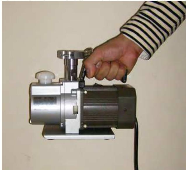
Fig. 5. A small rotary vacuum pump.
