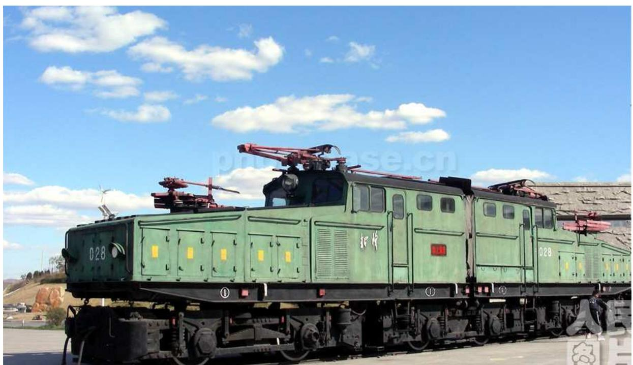
Fig. 2. Electrified train locomotive used in Haizhou Openpit mine.
