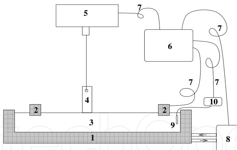
Fig. 1. A schematic diagram showing the experimental setup for the measurement of surface pressure ( $\pi$ ) - area per molecule ( $A_m$ ) isotherms. The basic parts of the setup are as follows: (1) teflon trough, (2) teflon barriers, (3) subphase (ion-free water), (4) Wilhemy plate (filter paper), (5) surface pressure sensor, (6) computer, (7) connecting wires, (8) thermostat, (9) resistance temperature detector (RTD) and (10) digital multimeter for measuring resistance
