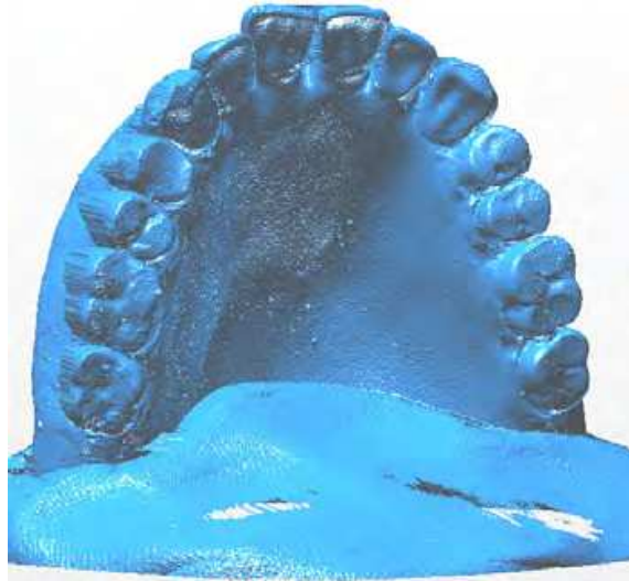
Fig. 4. The polygon mesh resulted from 3D scanning of the maxillary complete denture
