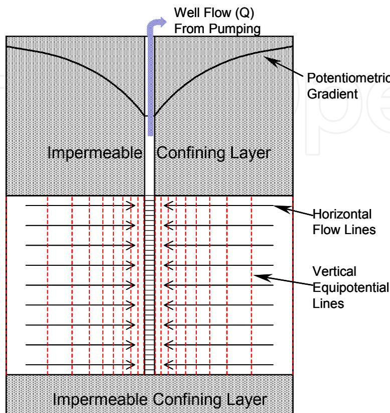
Fig. 1. Thiem equation for radial flow to wells. Equipotential lines are vertical and concentric about the well. Flow lines are horizontal and radial toward the well. The aquifer extends infinitely, and at infinity recharge equals well flow.
