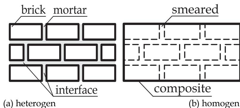
Fig. 2. Characterisation of masonry depending on the scale
