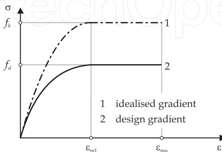
Fig. 3. Stress-Strain-Curve of masonry under compressive load
