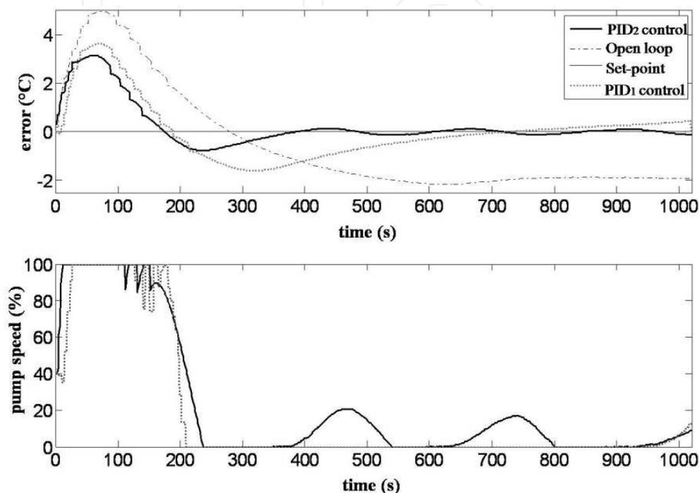
Fig. 4.4. Behavior of the controlled and manipulated variables under PID1 control ( $K_c=8\%/^{\circ}\text{C}$ ,  $\tau_i = 28\text{s}$  e  $\tau_d = 1,5\text{s}$ ) and PID2 ( $K_c=35\%/^{\circ}\text{C}$ ,  $\tau_i = 28\text{s}$  e  $\tau_d = 7\text{s}$ ).
