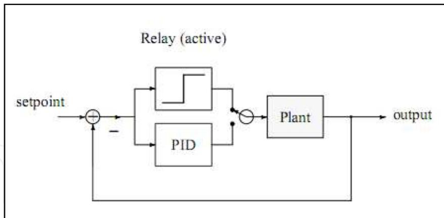
Fig. 3.1. Plant with the PID regulator temporarily disabled
