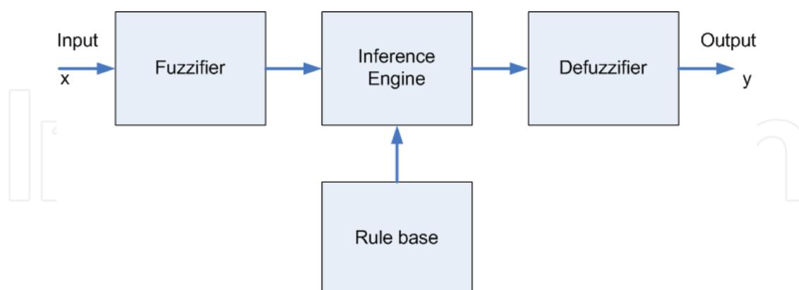
Fig. 6. Block diagram of a fuzzy inference system
