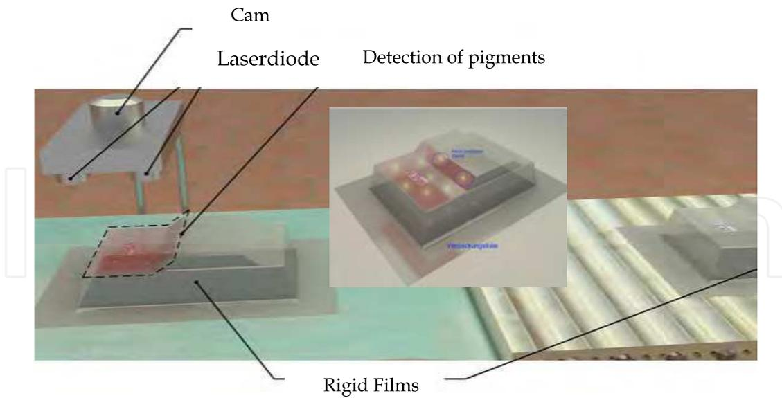
Fig. 14. Inline-Inspection system at the end of the calendaring process – shortly after the thermoforming-/ or the slitting process
