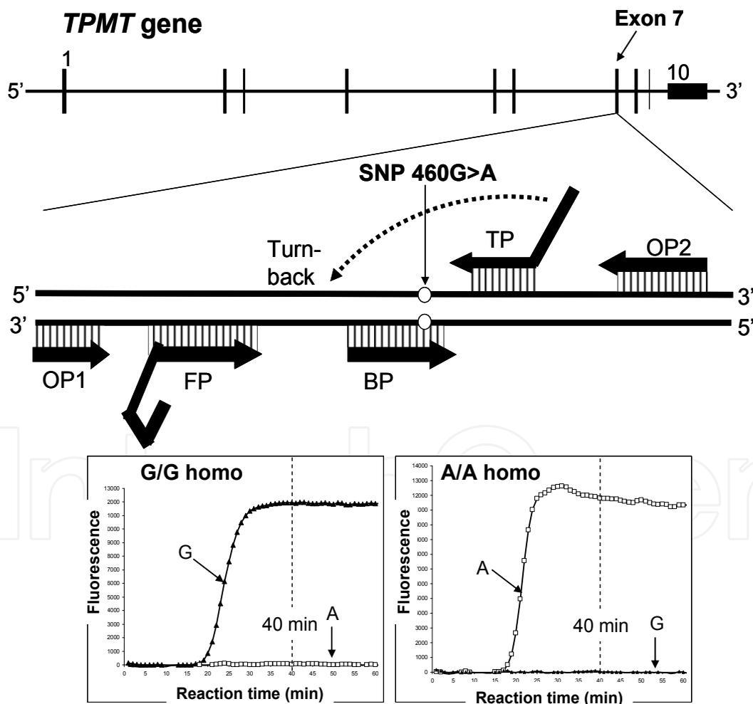
Fig. 5. Schematic illustration of the human *TPMT* gene and detection of the SNP 460G>A by the SmartAmp method. Two panels depict the time-courses of the SmartAmp assay reactions with *TPMT*-specific primers carrying WT (460G) or SNP (460A) alleles; namely, G/G homozygote and A/A homozygote.
