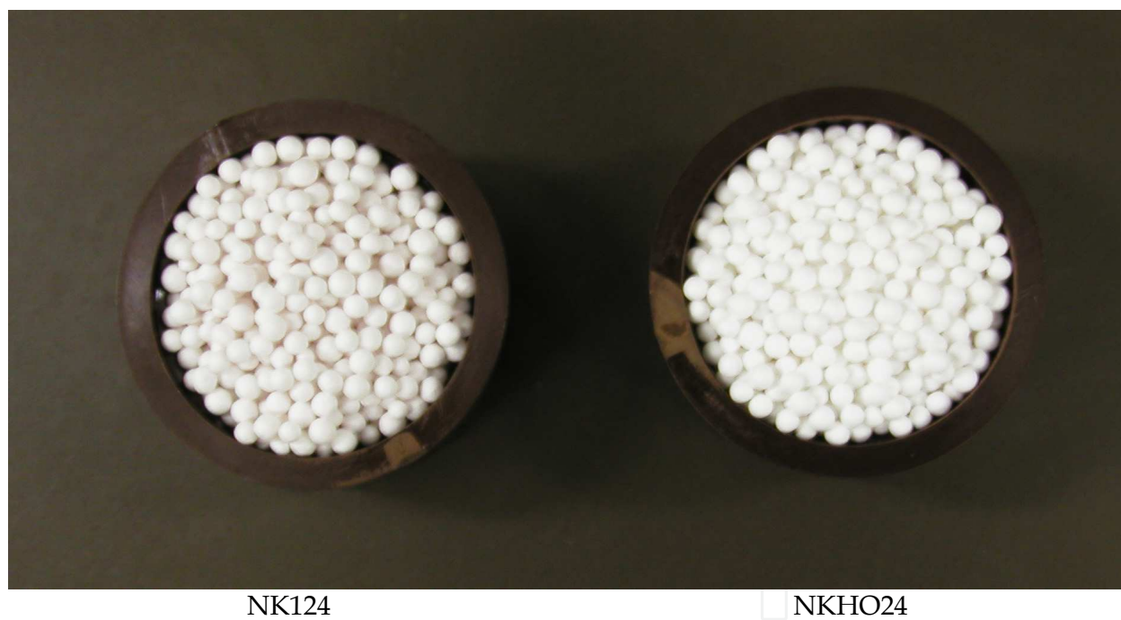
Fig. 2. Prepared alumina carrier-TiO 2 photocatalysts
