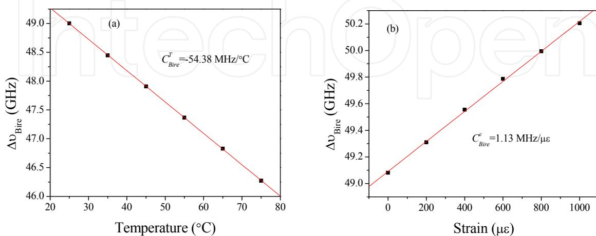
Fig. 17. The dependence of birefringence-induced frequency shift on (a) temperature and (b) strain. (Dong et al., 2010c, with permission from IEEE)
