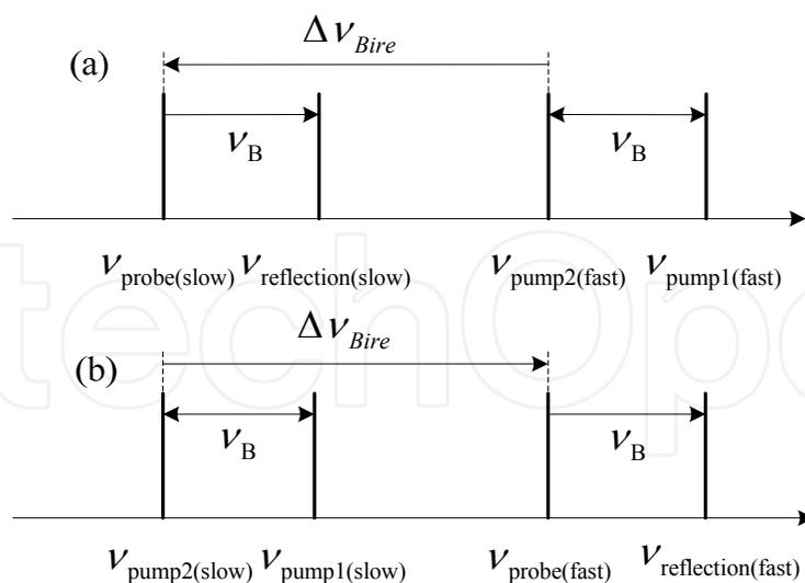
Fig. 15. Frequency relationship of pump1, pump2, probe and reflection: (a) the Brillouin grating is excited in the fast axis and probed in the slow axis, and (b) the Brillouin grating is excited in the slow axis and probed in the fast axis.
