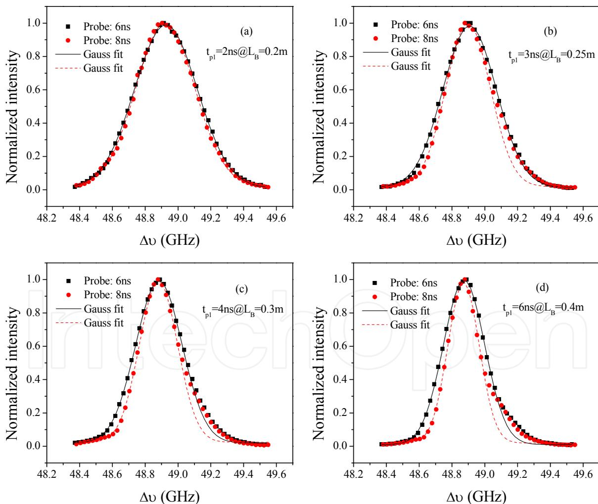
Fig. 12. Measured Brillouin grating spectra with 6 ns and 8 ns probe pulse with different pump 1 pulse-widths of (a) 2 ns, (b) 3 ns, (c) 4 ns, (d) 6 ns. Pump 2 pulse width is constant at 2 ns. (Dong et al., 2010b, with permission from OSA)
