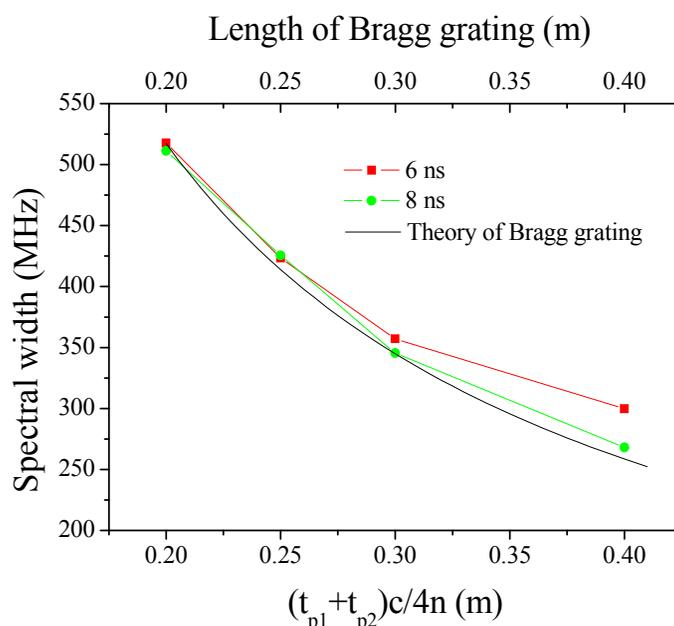
Fig. 13. The intrinsic Brillouin grating spectral width as a function of length. (Dong et al., 2010b, with permission from OSA)
