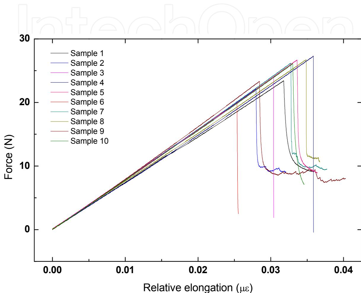
Fig. 2. Force versus strain experimental data for each sample of the standard optical fiber with the acrylate protective coating.
