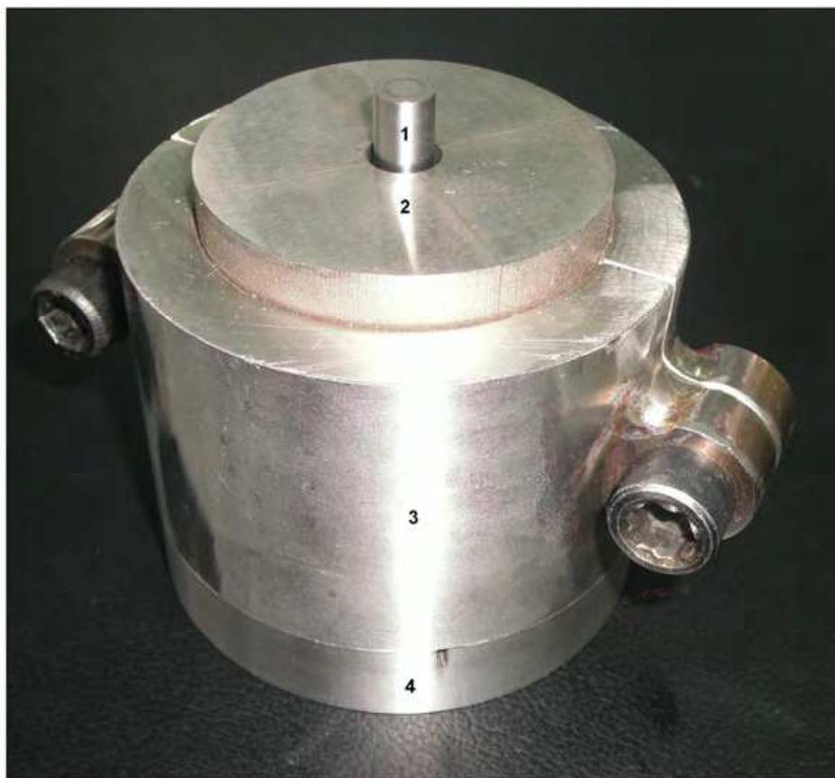
Fig. 2. The four-part dismantlable mold is shown in this picture: 1-punch, 2-four-section dismantlable block cylinder from high strength tempered steel, 3 - constricting clamp with two tightening bolts, 4 - support with groove for tungsten wire.
