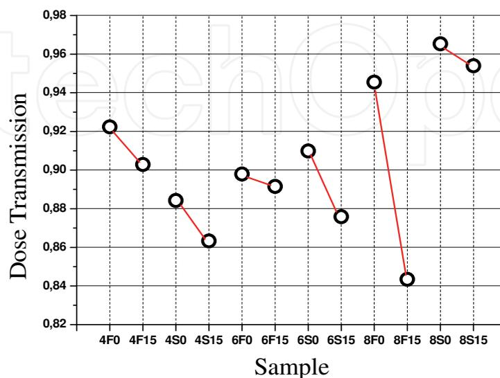
Fig. 5. 4.5 MeV neutron dose transmissions for each samples
