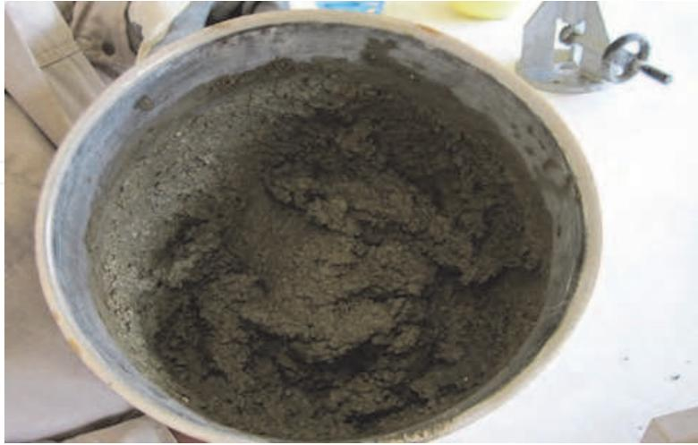
Fig. 2. Fresh state of lightweight mortar prepared with expanded vermiculite aggregate.
