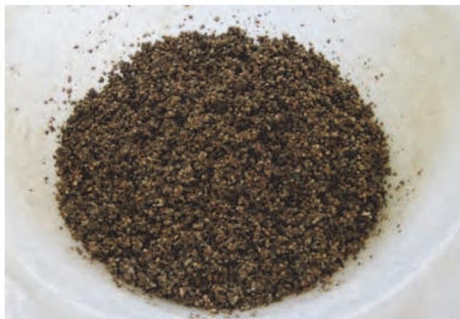
Fig. 1. Expanded vermiculite fine aggregate saturated with water.
