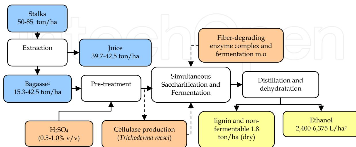
Fig. 3. Flowchart for ethanol production from sweet sorghum bagasse. <sup>1</sup> Average composition of sweet sorghum bagasse: Water 54%, simple fermentable sugars 5.4%; Cellulose 17%; Hemicellulose 12%; Lignin 11.7% <sup>2</sup> Practical yield from fermentation with *I. orientalis*: 3,865 L/ha. From: Almodares & Hadi (2009); Gnansounou et al. (2005).
