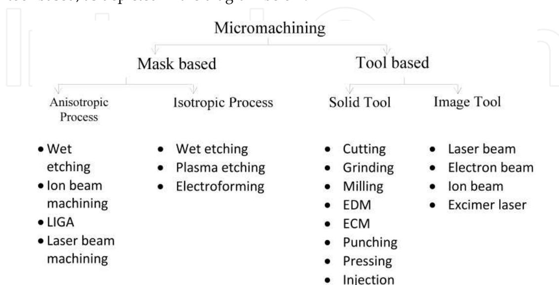
While mask-based processes can generate 2-D/2.5-D features on substrates like semiconductor chips, tools-based processes have the distinct advantage of being able to adapt to metallic and non-metallic surfaces alike, and also generate 3-D features and/or free-form sculpted surfaces. However, the challenges of achieving accuracy, precision and resolution persist.
