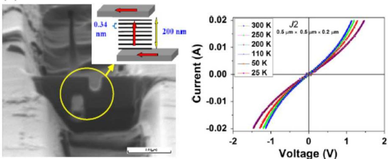
Fig. 4. FIB image of the nanoscale stack fabricated on a thin graphite flake along the *c*-axis height of 200 nm (image scale bar is 2  $\mu\text{m}$ ). Inset shows the schematic diagram of stack arrangement along the *c*-axis. (Venugopal et al, 2011). The vertical red arrow indicates the current flow direction through the nanoscale stack.  $I$ - $V$  characteristics at various temperatures of the fabricated nanostack are also shown (right).
