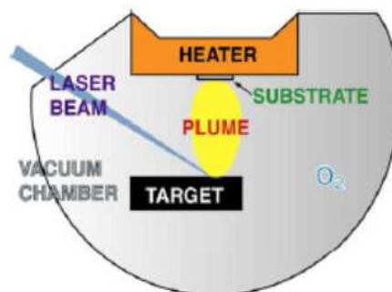
Fig. 2. Laser ablation experiment.
