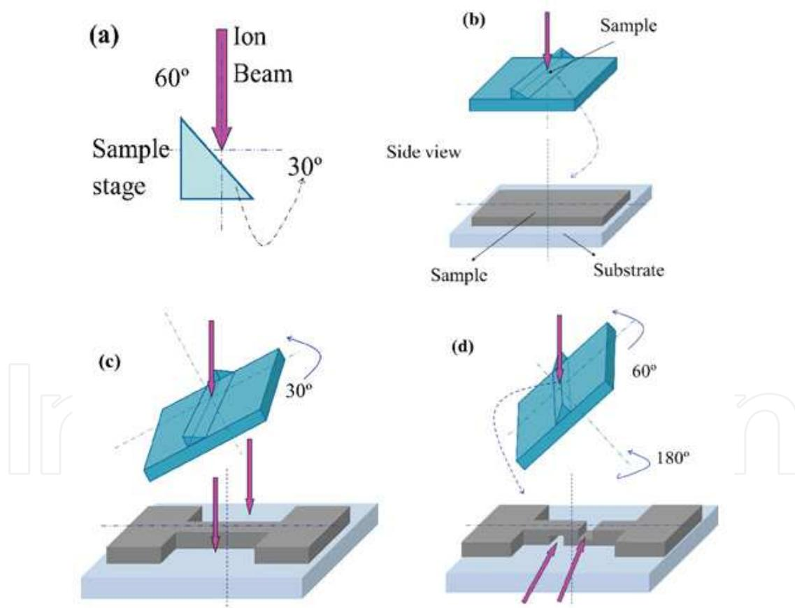
Fig. 3. FIB 3-D fabrication process (a) Scheme of the inclined plane has an angle of  $60^\circ$  with ion beam (where we mount sample). (b) The initial orientation of sample and sample stage. (c) Sample stage tilted by  $30^\circ$  anticlockwise with respect to ion beam and milling along *ab*-plane. (d) The sample stage rotated by an angle of  $180^\circ$  and also tilted by  $60^\circ$  anticlockwise with respect to ion beam and milled along the *c*-axis.
