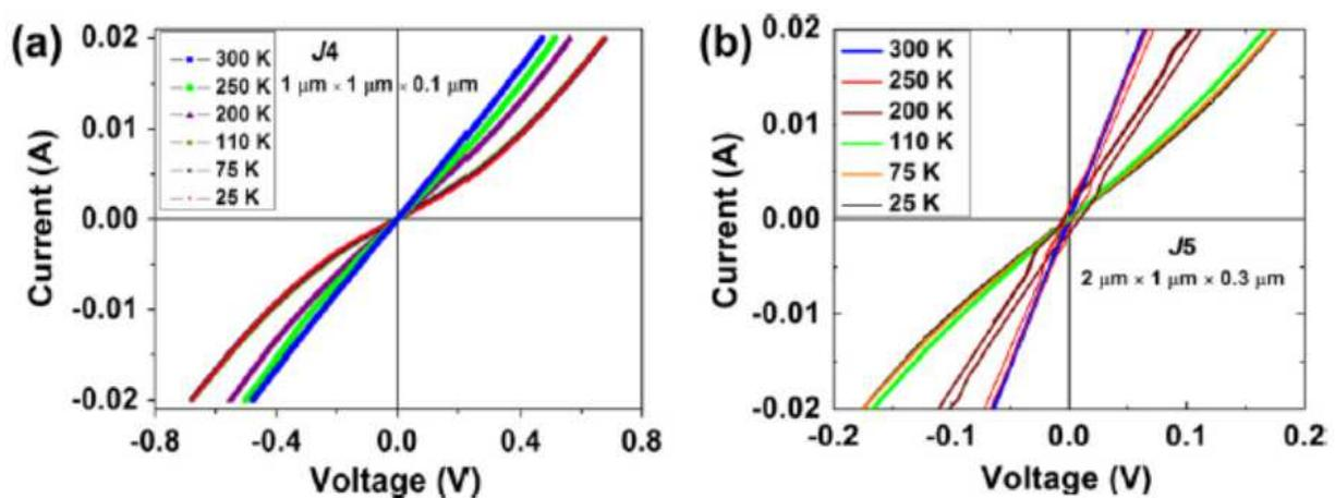
Fig. 5. (a)  $I$ - $V$  characteristics of a bigger stacked-junction with  $A$  of  $1 \mu\text{m}^2$  ( $J4$ ) at different temperature from 25 K to 300 K. (b)  $I$ - $V$  characteristics of another bigger junction with  $A$  of  $2 \times 1 \times 0.3 \mu\text{m}^3$  ( $J5$ ) at different temperature from 25 K to 300 K. Both the junctions show ohmic like behavior at 300 K; however the same behavior turned into nonlinear characteristics when the temperature goes down (Venugopal et al, 2011).
