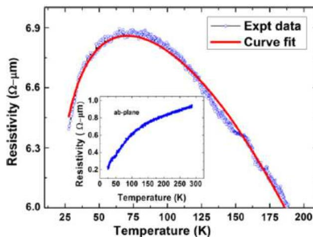
Fig. 6. The resistivity-temperature ( $\rho$ - $T$ ) characteristics of nanostack which shows a clear  $c$ -axis characteristics of graphite. A well agreed curve fitting to experimental data is also shown. A clear metallic behavior is observed for  $ab$ -plane transport of bare graphite flake which is shown as inset. (Venugopal, 2011)
