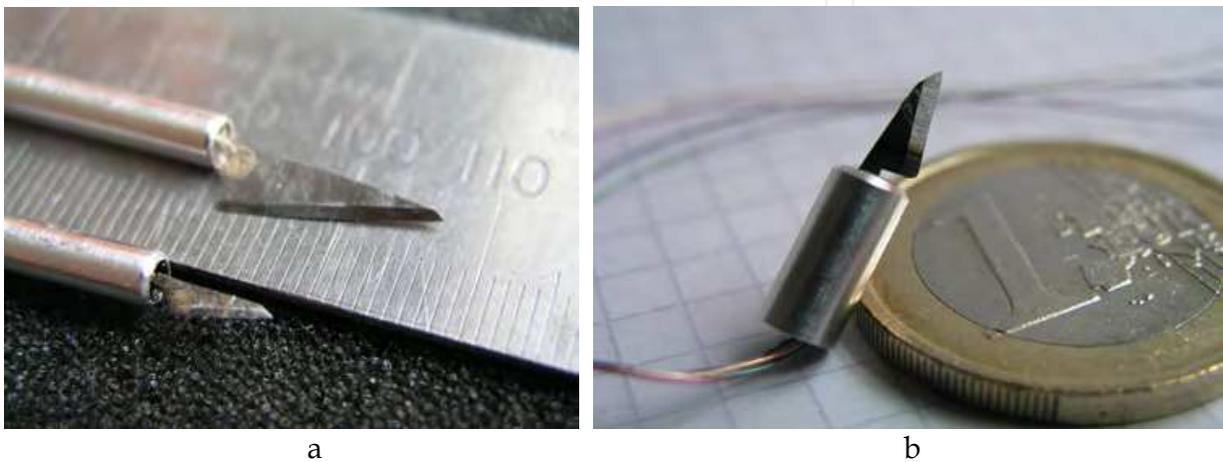
Fig. 5. a. Prototypes with an overall length of 25 and 50mm including the support structure; b. Prototype of total length 20 mm
