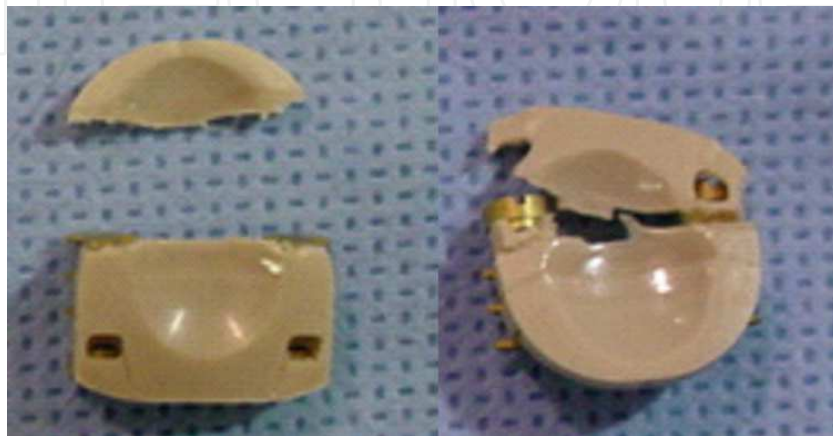
Fig. 2. PEEK cervical arthroplasty device after static compressive shear testing to failure. Left – tested under 10° flexion, right – tested under 10° extension.
