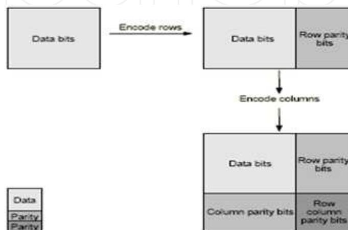
Fig. 1. Regular Product Code Encoding Procedure.
