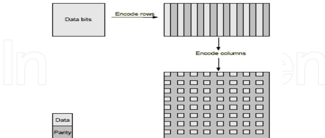
Fig. 3. CPC Encoding Procedure without an Interleaver.
