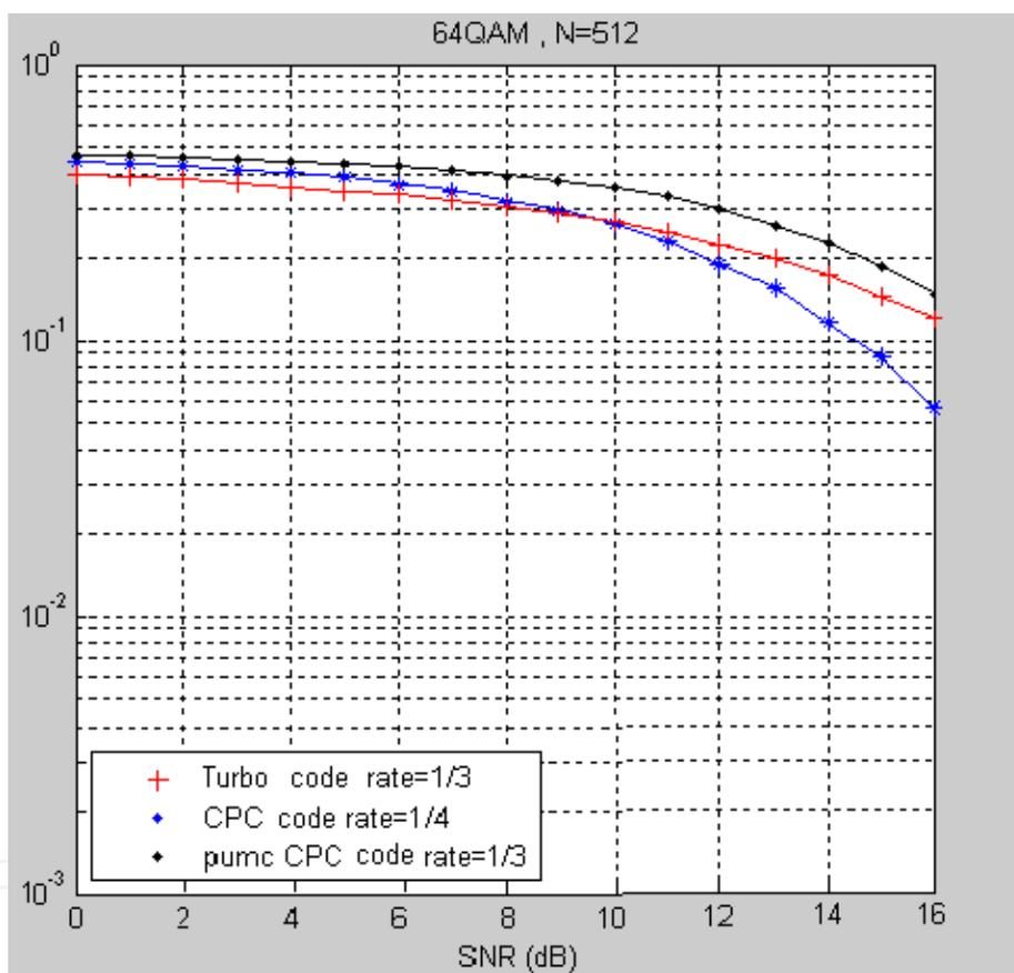
Fig. 43. BER Comparison between Turbo code, CPC, punctured CPC at 64 QAM, N=512.
