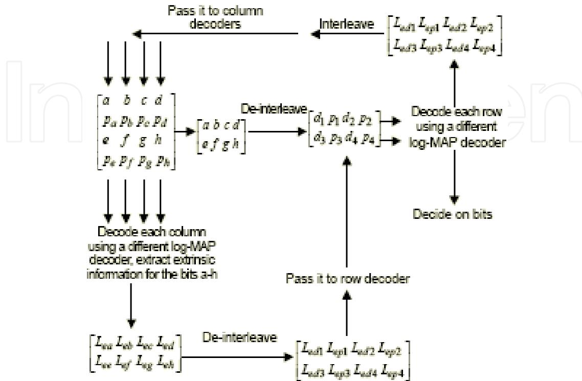
Fig. 5. Decoding Operation of the Convolutional Product Code.
