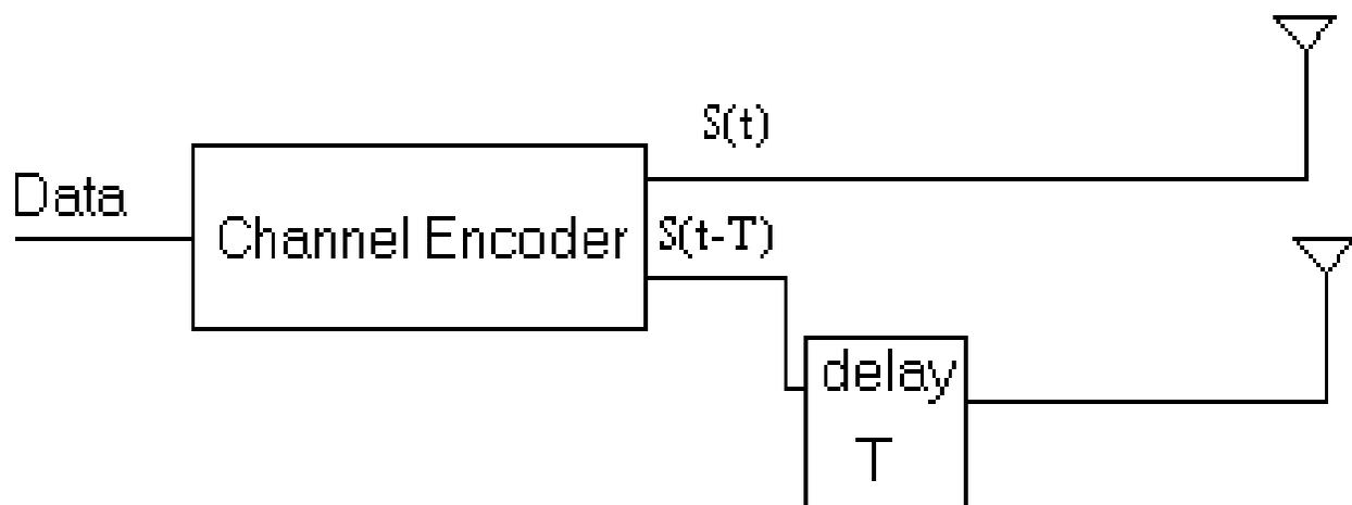
Fig. 44. Transmit Delay Diversity Scheme
