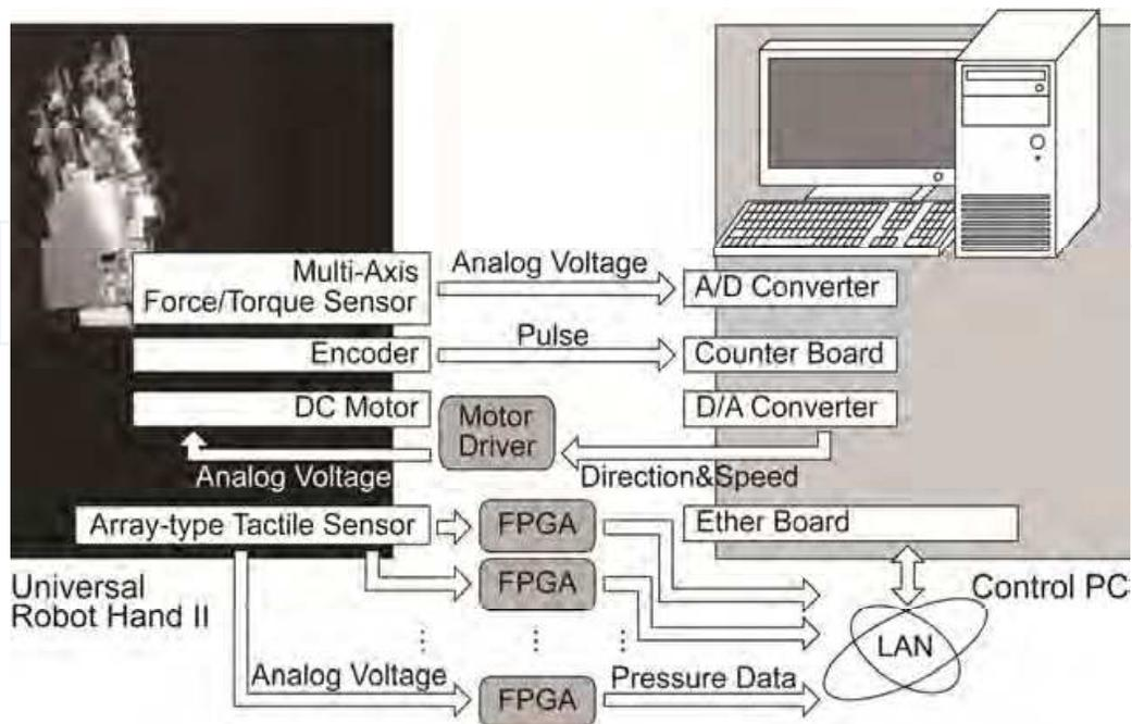
Fig. 4. Control system for universal robot hand
