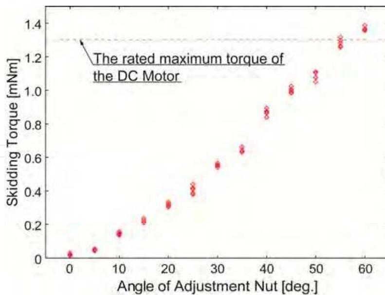
Fig. 8. Angle of adjustment nut vs skidding torque
