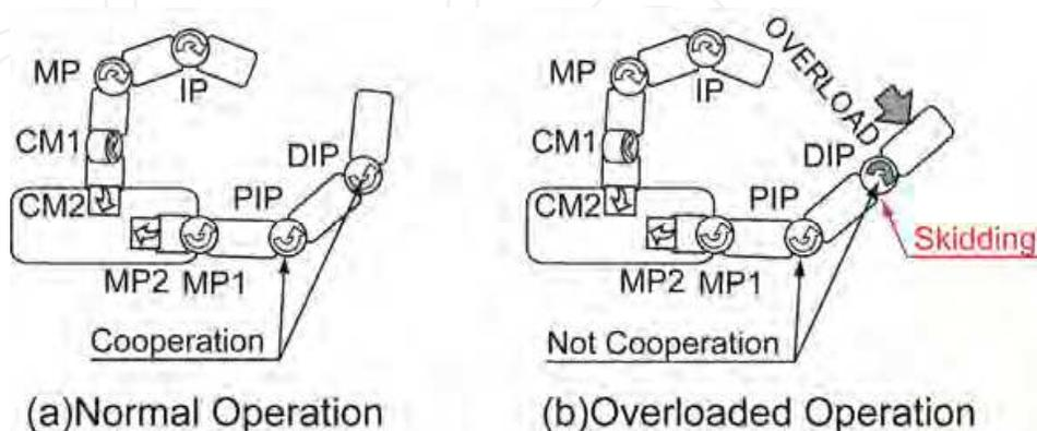
Fig. 9. Overloaded operation with torque limiter mechanism
