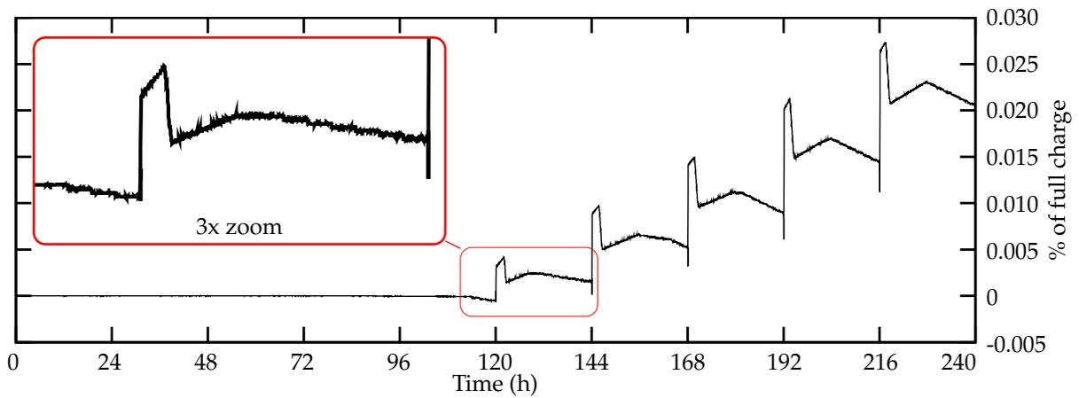
(b) Difference in the average energy in nodes for simulations in  $S_1$ . Given that the two curves in Fig. 11(a) are characterised by the functions  $f_{\text{DEHAR}}(t)$  and  $f_{\text{DD}}(t)$ , then the curve in this figure is characterised by  $f_{\text{DEHAR}}(t) - f_{\text{DD}}(t)$ .
