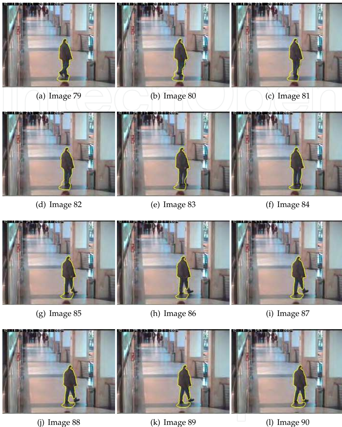
Fig. 12. Detection and tracking of a non-rigid dynamic object along 12 consecutive images. In each image, 30 iterations are used in order to find the object silhouette.
