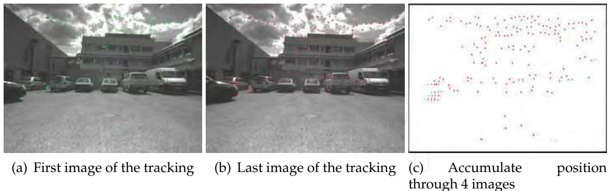
Fig. 6. N feature points initially detected at image a) are tracked through 4 images. Image b) displays the last image during the tracking task. Image c) depicts all the accumulate positions for the N initial points detected calculated by the tracking process.
