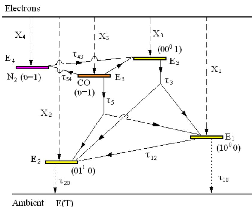
Fig. 3. Schematic energy-level diagram for N<sub>2</sub>-CO<sub>2</sub>-CO system
