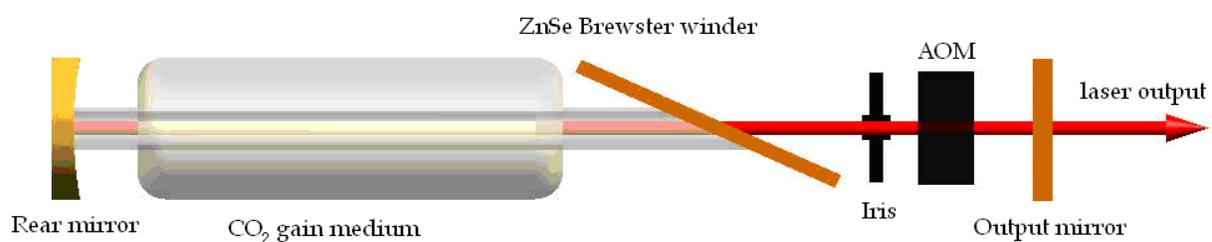
Fig. 2. Schematic diagram of acousto-optically Q-switch CO<sub>2</sub> laser
