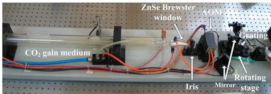
Fig. 16. Tunable acousto-optically Q-switch CO<sub>2</sub> laser
