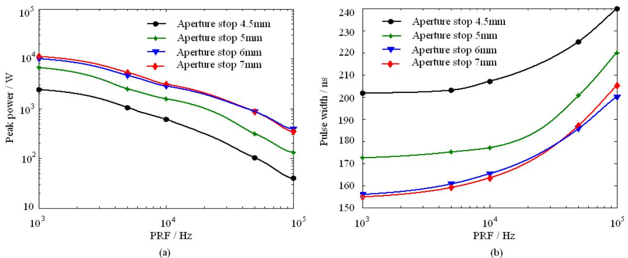
Fig. 11. Peak power (a), pulse width (b) of the CO<sub>2</sub> laser as a function of apertures stop
