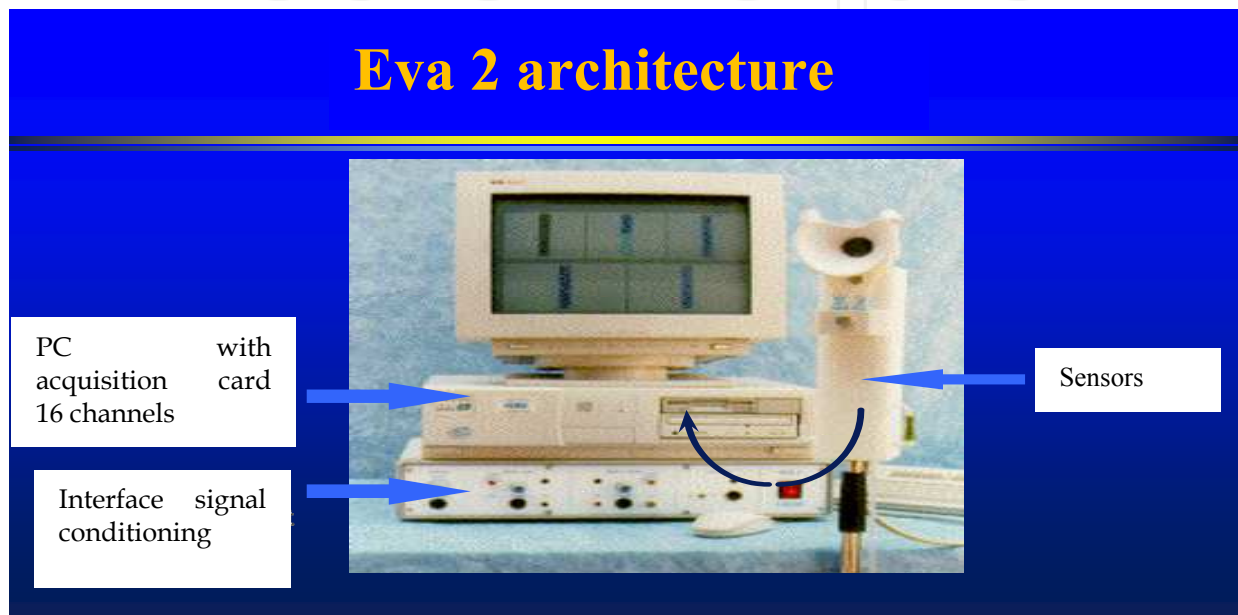
Fig. 1. General Feature of Eva 2 (workstation PC in the Windows environment)
