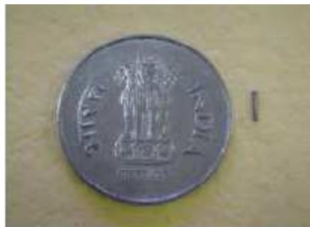
Fig. 7. Encapsulated  $^{125}\text{I}$ - brachytherapy sources
