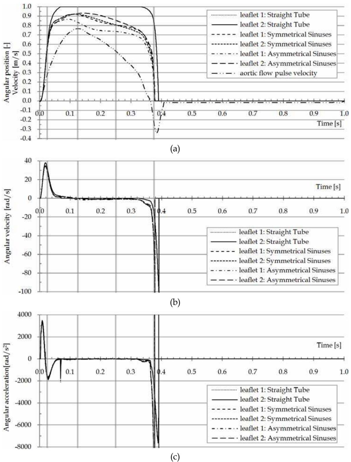
Fig. 4. Angular position of the leaflets (relative to maximal opening angle) and the aortic flow pulse velocity (a), angular velocity of the leaflets (b) and angular acceleration of the leaflets (c). The two leaflets of the geometry with the straight tube perform a complete symmetrical movement. The time levels at which the contours in Fig. 5 are shown are visualized by the vertical lines
