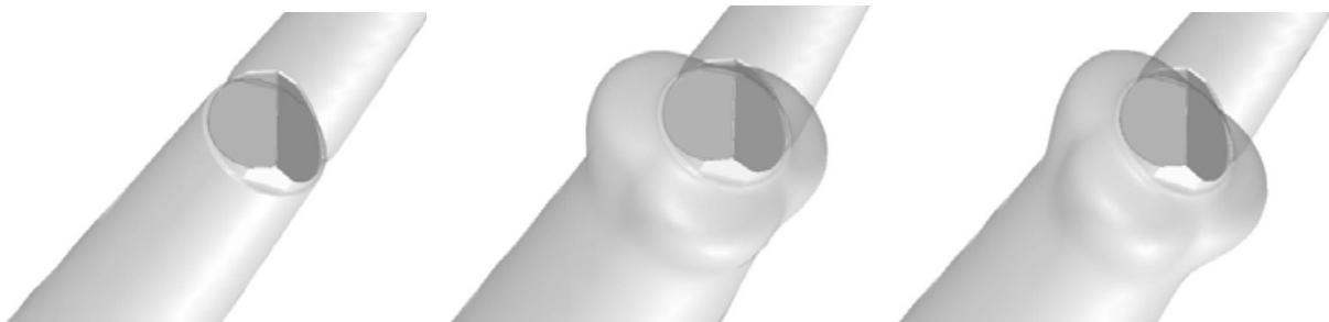
Fig. 3. Isometric view of the different geometries. *Left*: first geometry with straight tube. *Middle*: second geometry with symmetrically placed sinuses of Valsalva. *Right*: third geometry with asymmetrically positioned sinuses of Valsalva downstream of the valve
