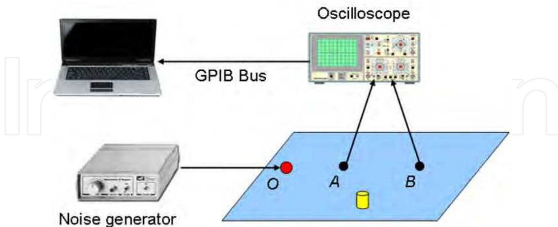
Fig. 11. Experimental set-up for defect detection.
