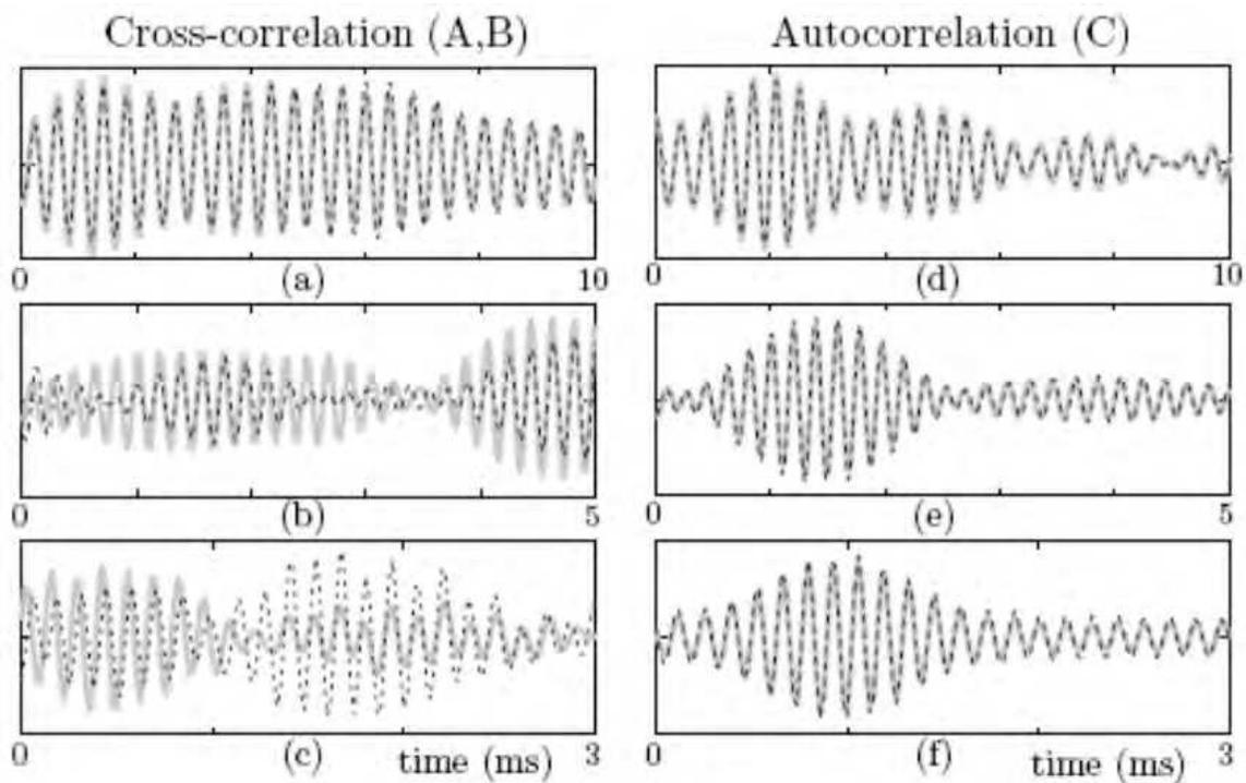
Fig. 15. Filtered average cross-correlation (a, b, c) and autocorrelation (d, e, f) functions with (broken line) and without (solid line) defect. (a), (d)  $f_0 = 2.5$  kHz,  $N = 10$  cycles. (b), (e)  $f_0 = 5.2$  kHz,  $N = 15$  cycles. (c), (f)  $f_0 = 7.8$  kHz,  $N = 15$  cycles.
