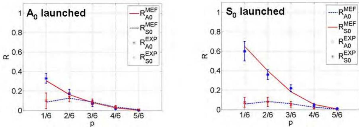
Fig. 6. Comparison between numerical and experimental results for the reflection (R) coefficient, when the launched Lamb mode A<sub>0</sub> (a) or S<sub>0</sub> (b) interacts with an asymmetrical discontinuity.
