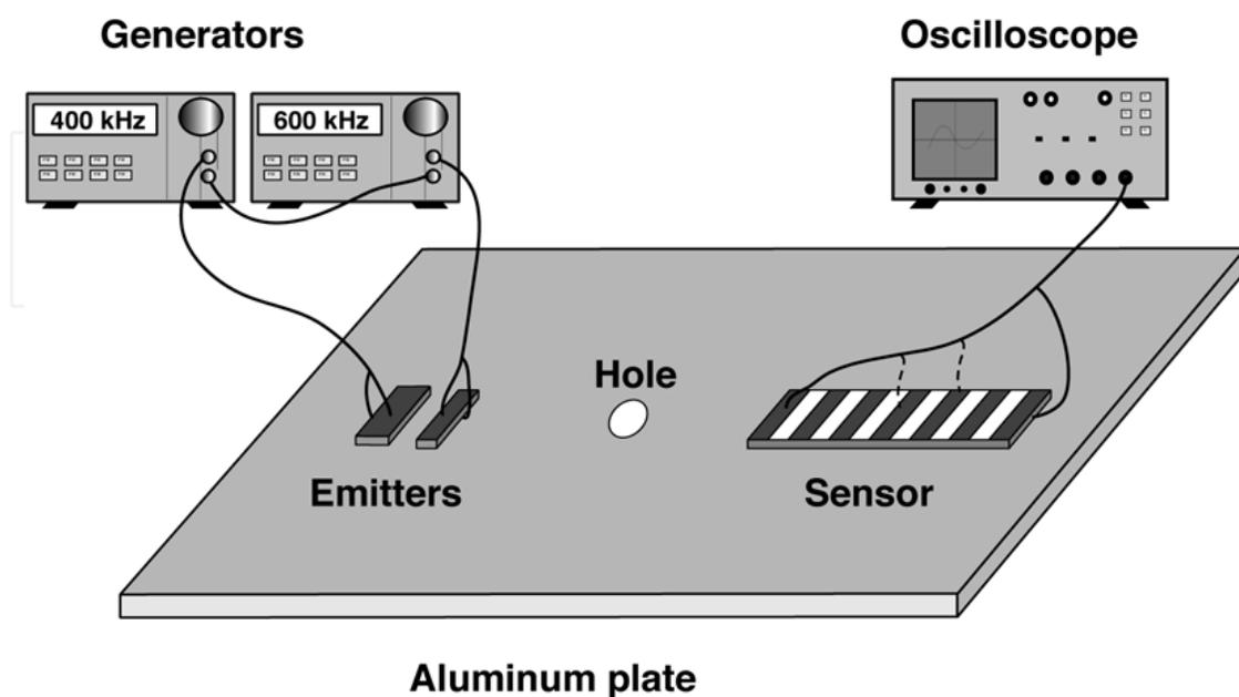
Fig. 7. Experimental measurement setup
