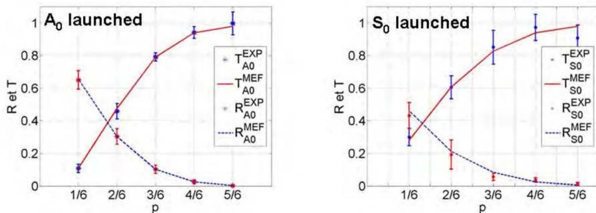
Fig. 5. Comparison between numerical and experimental results for the reflection (R) and the transmission (T) coefficients, when the launched Lamb mode  $A_0$  (a) or  $S_0$  (b) interacts with a symmetrical discontinuity.
